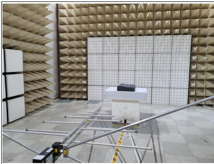
**3. Photo of Radiated Spurious Emission Test (Above 1 GHz)**
