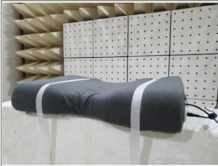
**2. Photo of Radiated Spurious Emission Test (Below 1 GHz)**
