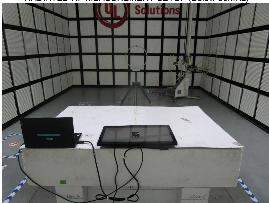
RADIATED RF MEASUREMENT SETUP (Below 30MHz)
