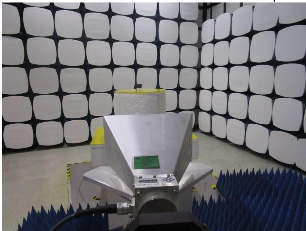
**1.3 Radiated Spurious Emissions Test setup**
