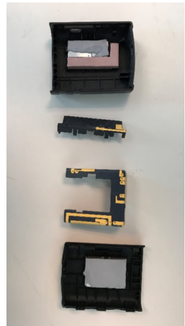
EUT Antenna and cover
