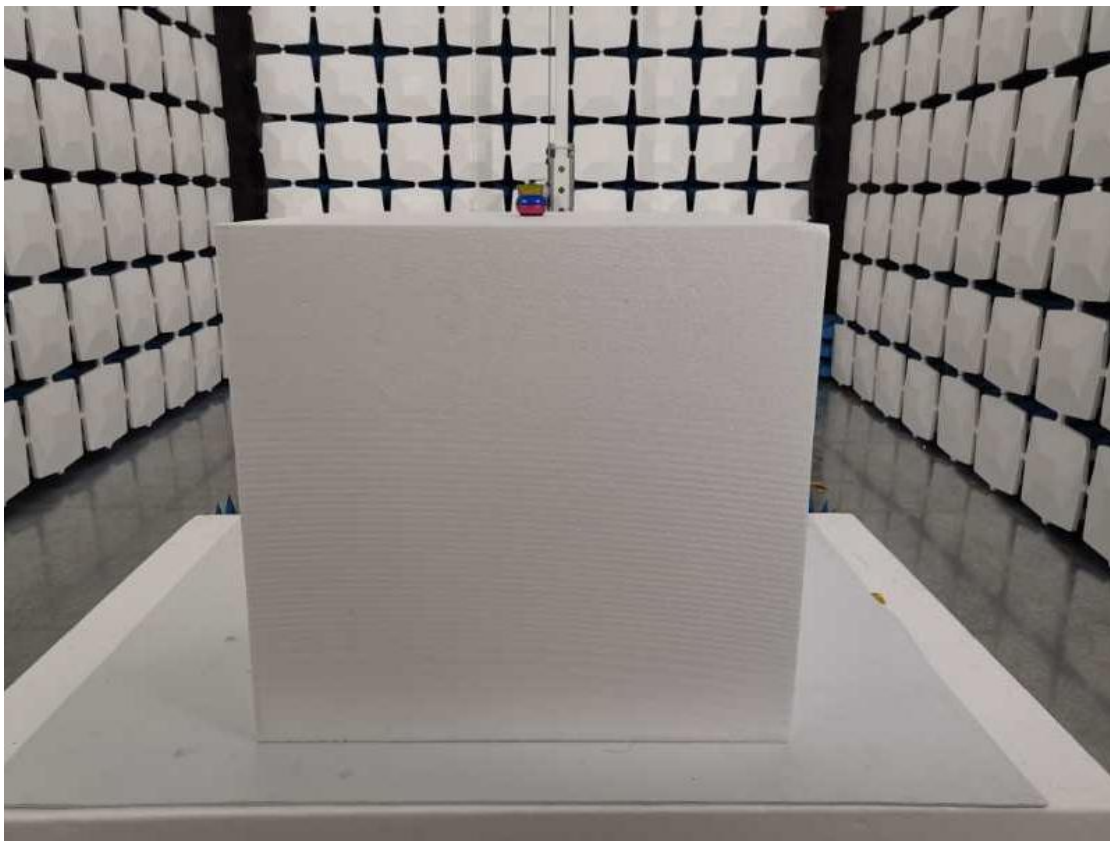
Above 1GHz for radiated emission test setup
