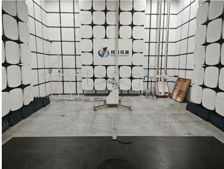
Radiated Spurious Emissions From 30MHz-1000MHz
