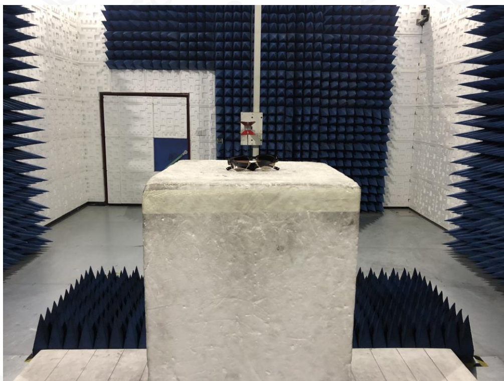
RADIATED EMISSION TEST SETUP ABOVE 1GHZ
