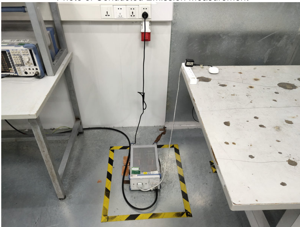
FCC ID: 2AV49-KH-30 Photo of Conducted Emission Measurement
