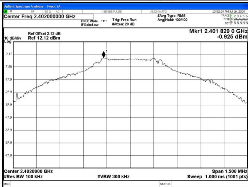
Tx. Spurious NVNT 1-DH5 2402MHz Ant1 Emission
