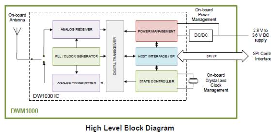
The DWM 1000 module is based on Decawave's DW 1000 Ultra Wideband (UWB) transceiver IC. It integrates antenna, all RF circuitry, power management and clock circuitry in one module. It can be used in 2-way ranging or TDOA location systems to locate assets to a precision of 10cm and supports data rates of up to 6.8 Mbps
