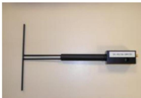
Figure 1 – Satimo COMOSAR Validation Dipole
