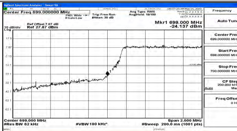
Band Edge Test Graph(s) (Channel Bandwidth: 1.4 MHz)_LCH_16QAM
