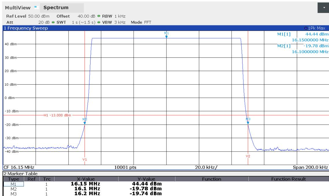
Frequency band: 16.100 MHz to 16.200 MHz; EUT is in ID mode
