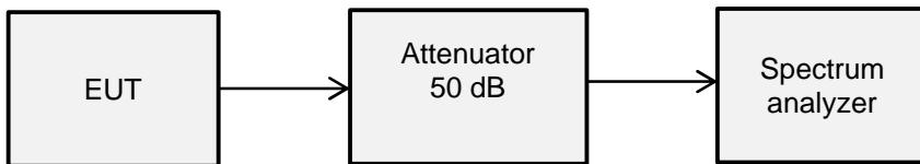
The following spectrum analyser settings for band edge measurements were used:
