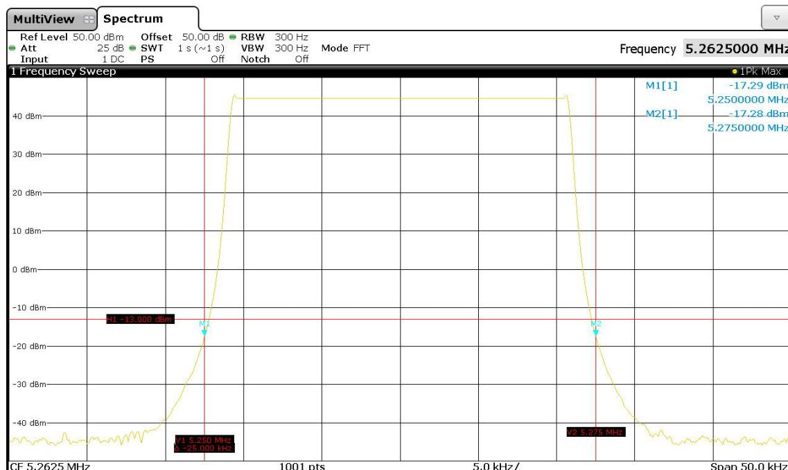
Frequency band: 5.250 MHz to 5.275 MHz; EUT is ID mode
