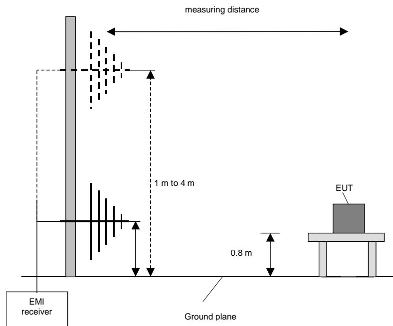
For the final measurement the highest emissions, closest to the limit line will be selected. For each emission a continuous partial scan for 1 m antenna height and 50° azimuth at the turntable will be performed, to determine the worst case.
