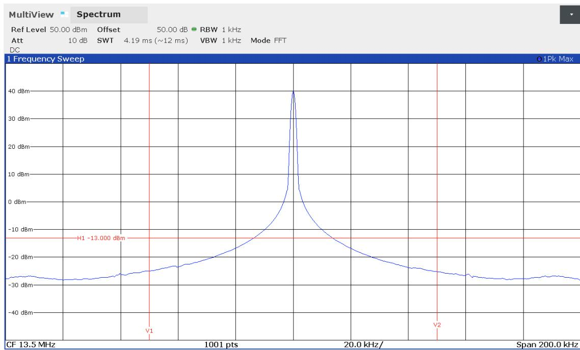
Frequency band: 16.100 MHz to 16.200 MHz; EUT in sweep mode
