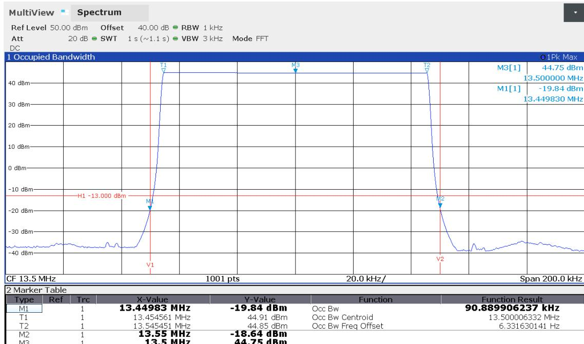
Frequency band: 13.450 MHz to 13.550 MHz; EUT is in ID mode
