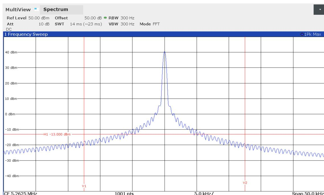
Frequency band: 13.450 MHz to 13.550 MHz; EUT in sweep mode
