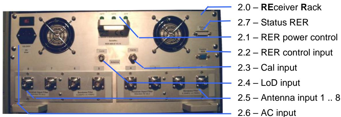
Figure 3.1: Back view, WERA RER internal Filters (8 channels)
