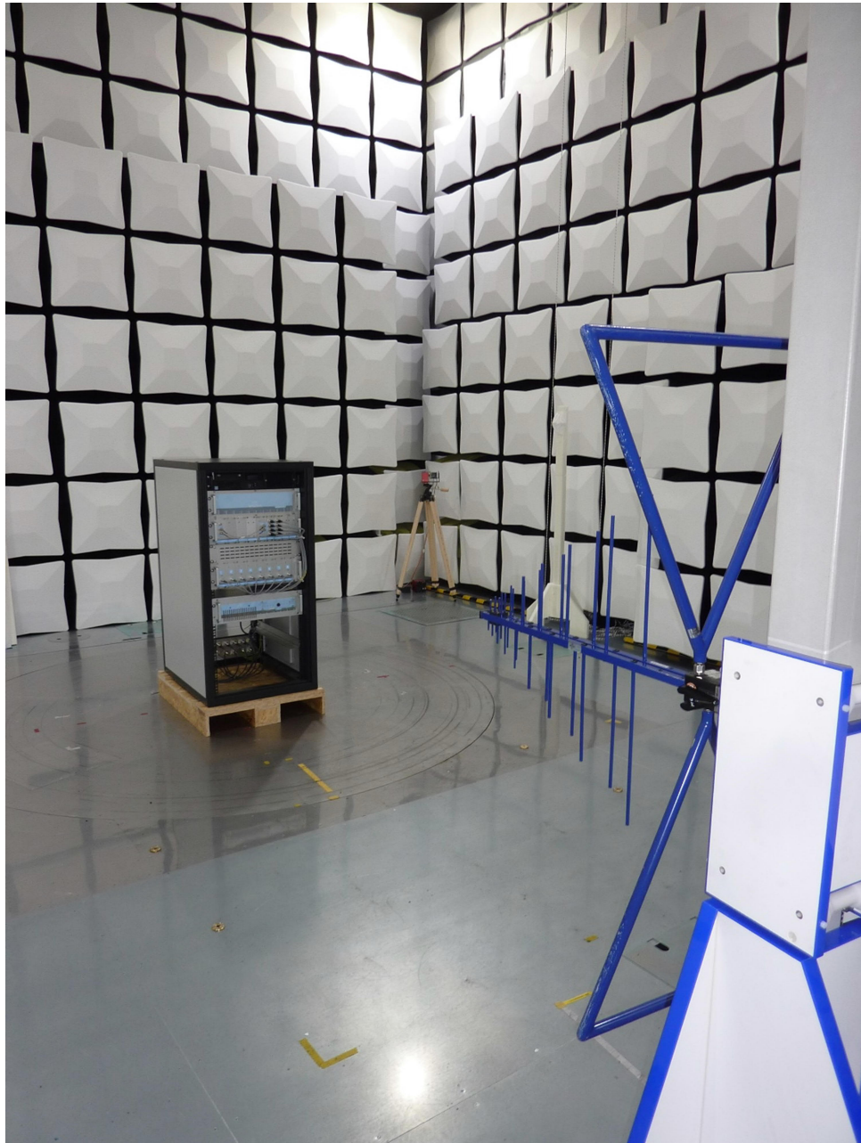
Test setup semi anechoic chamber 30 MHz – 1 GHz
