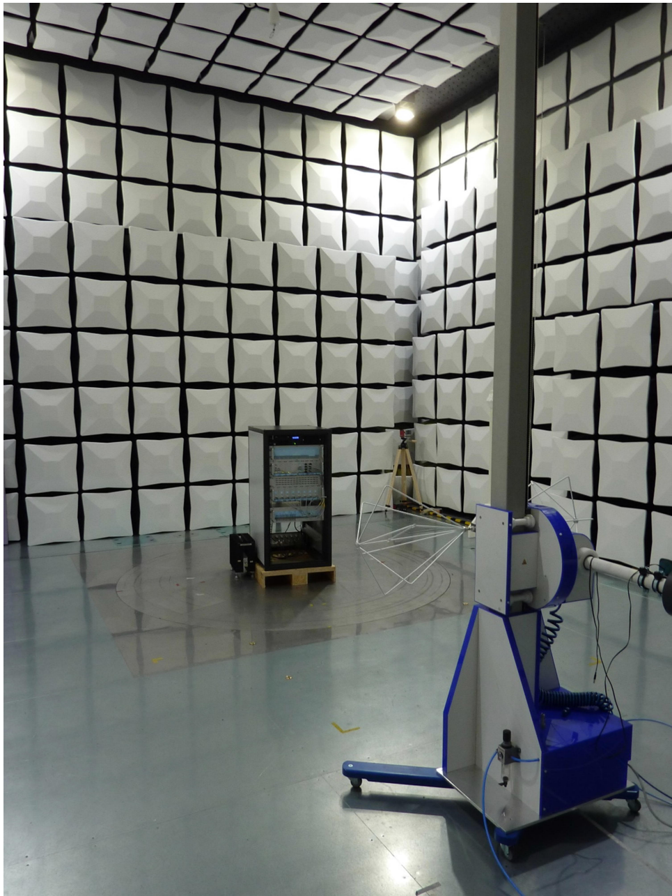
Test setup semi anechoic chamber 30 MHz – 200 MHz
