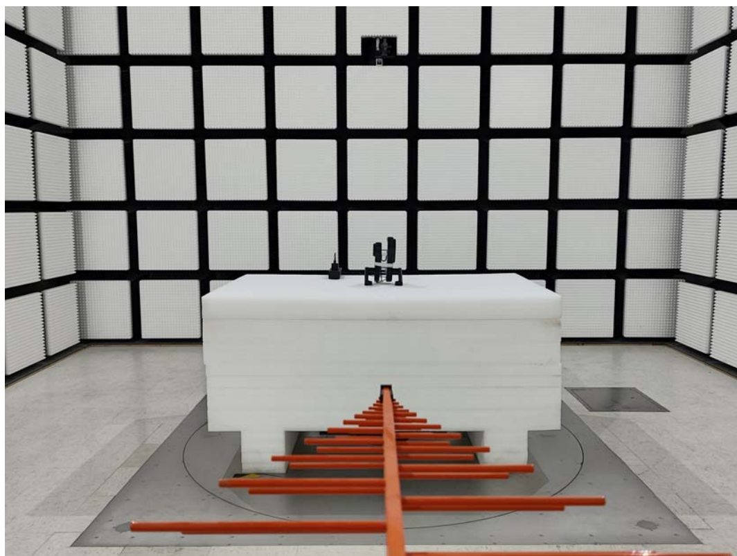
Radiated Emission Above 1GHz View
