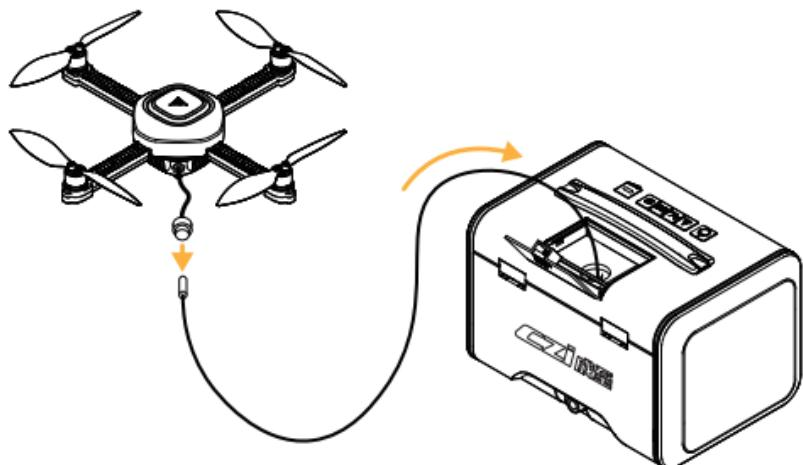
11. Place the Airborne unit into its protective sleeve and return it to the Ground Station. Close the cover.
