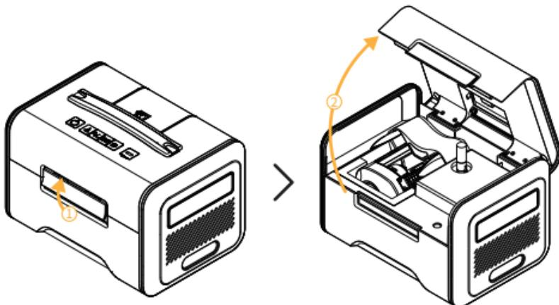
4. Remove Airborne unit from Ground Station and unfold.
