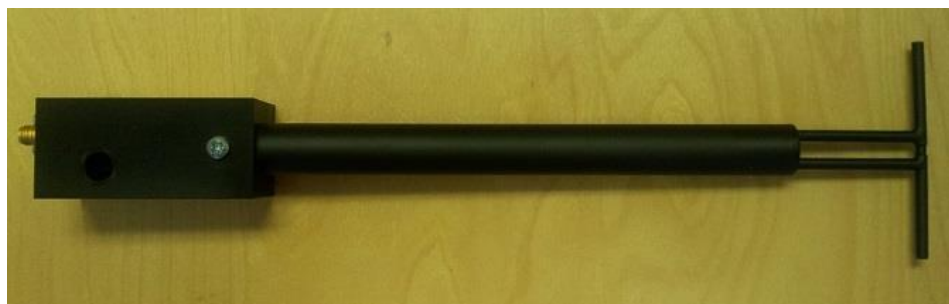
Figure 1 – MVG COMOSAR Validation Dipole
