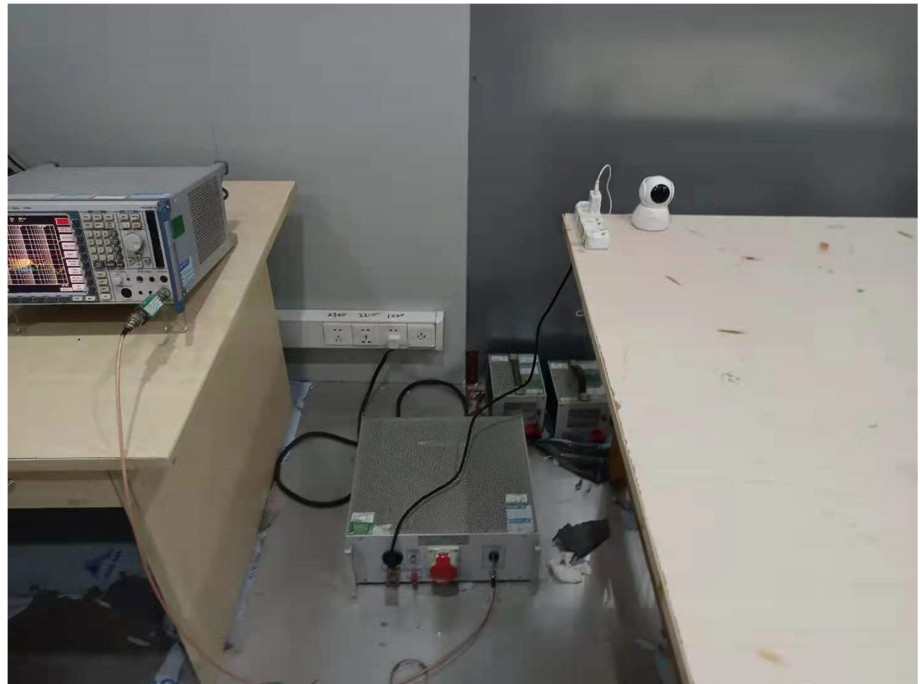
Conducted Emission Test Setup
