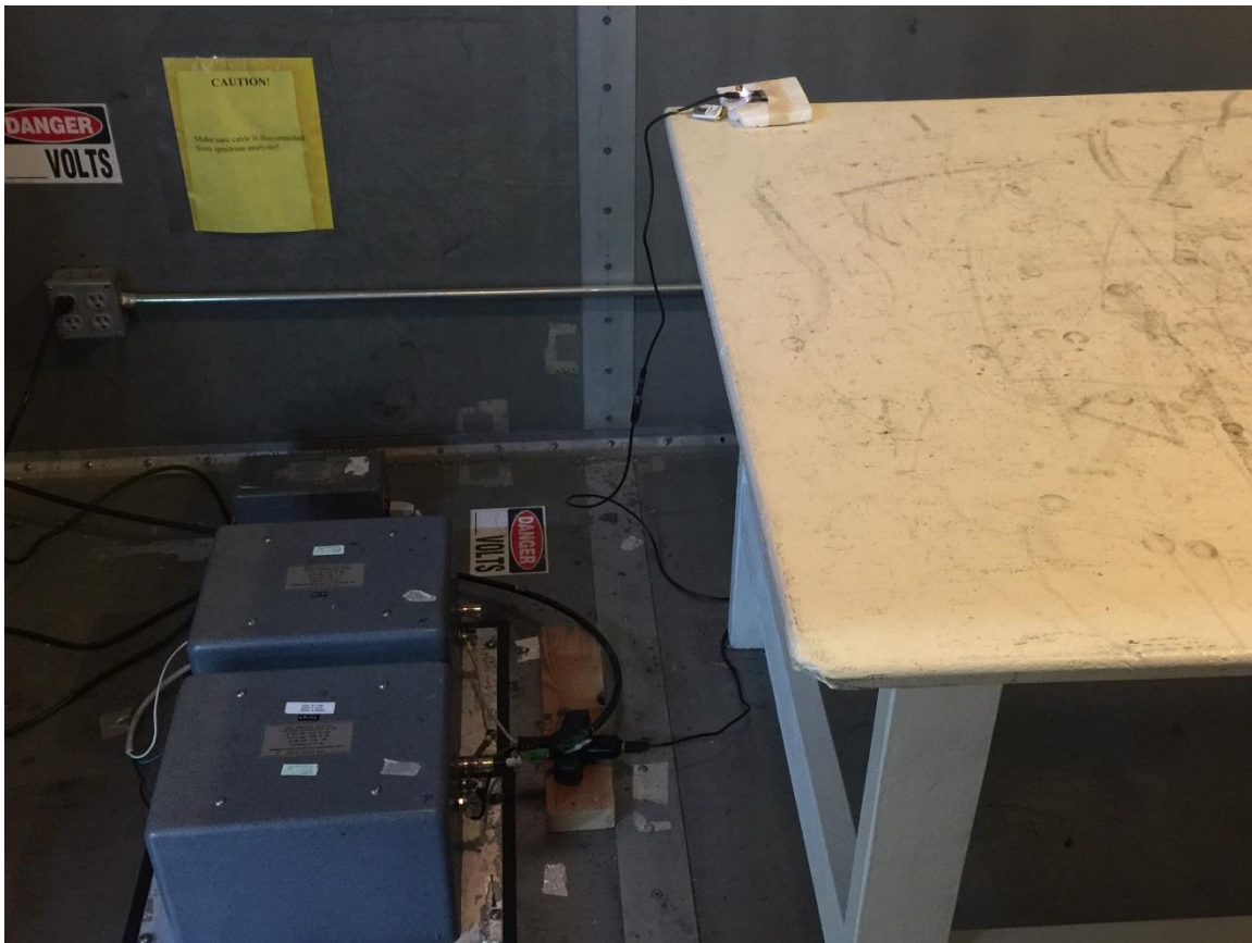
PHOTO 7. CONDUCTED EMISSION TEST SETUP
