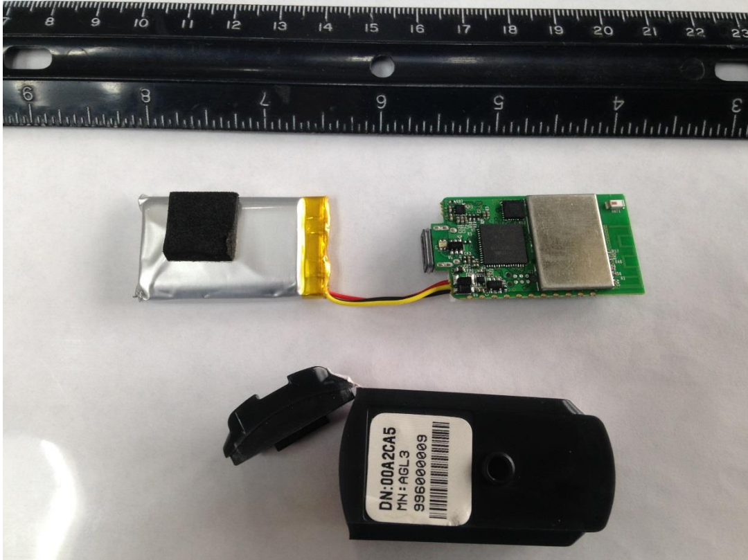
Photo 1. EUT with Battery Pack, Removed from Enclosure
