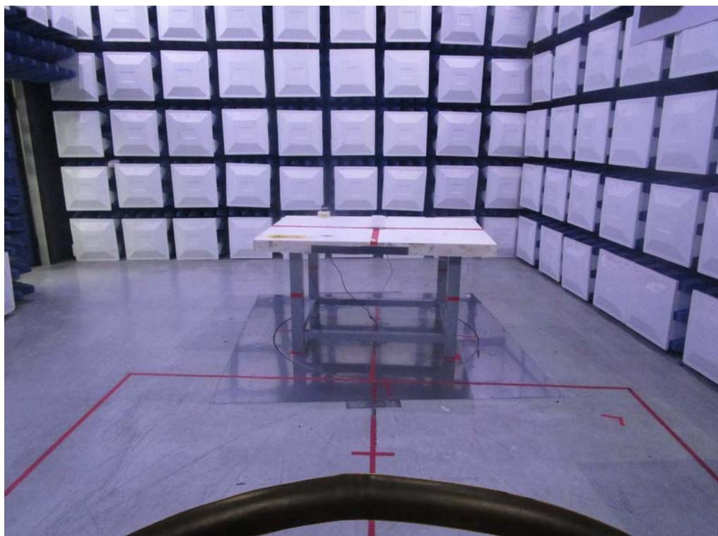
**Radiated Emissions Test Photos****30 MHz to 1 GHz**
