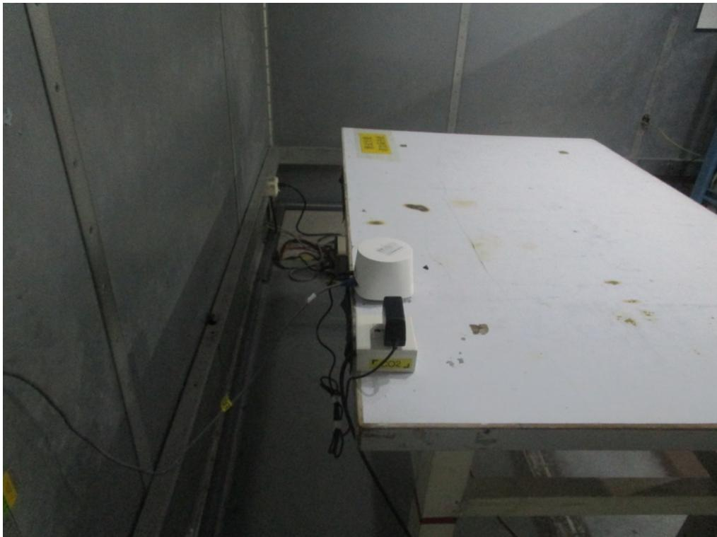
**Radiated Emissions Test Photos****9 kHz to 30 MHz**
