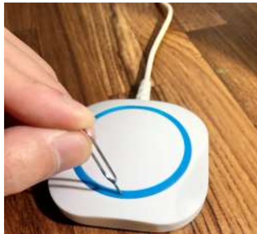
Figure 4. Press the reset button to reset the mattress data gateway
