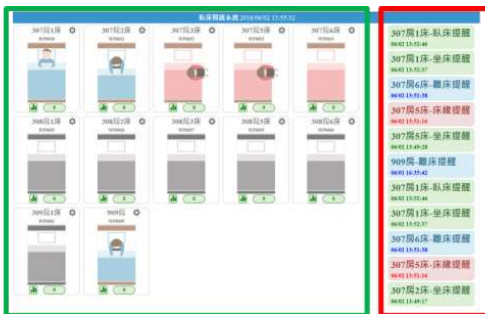
Figure 6. The multi-person monitoring UI for the bed status and bed exit event.
