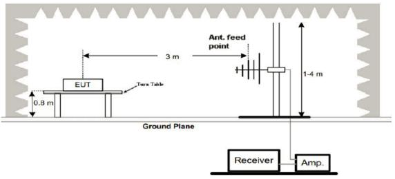
(3) Radiated Emission Test-Up Frequency Above 1GHz
