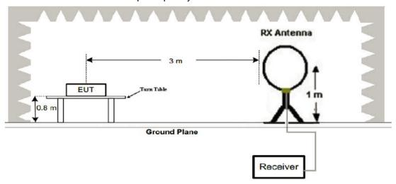
(2) Radiated Emission Test-Up Frequency 30MHz~1GHz
