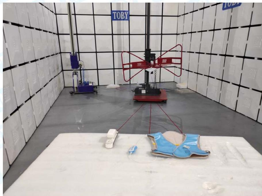
**Photo of Setup for Conducted Emission**
