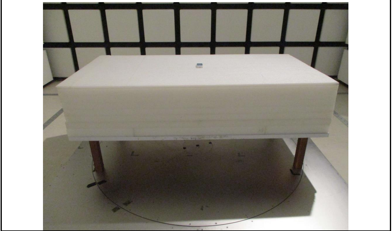
Radiated Emission Below 1GHz Test
