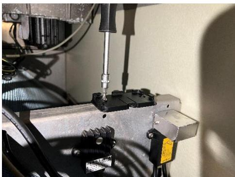
15. Slide the transceiver into the bracket so it clicks into place.
