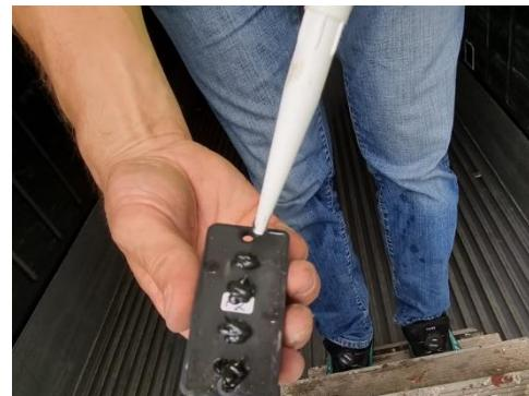
7. Ensuring that the arrows on the label or the flat side of the sensor point out to the container door, use a screwdriver and 2 screws to mount the sensor. If using glue, press the sensor firmly into position and hold it there for 1 minute before applying some tape to hold it in place while the glue is drying.
