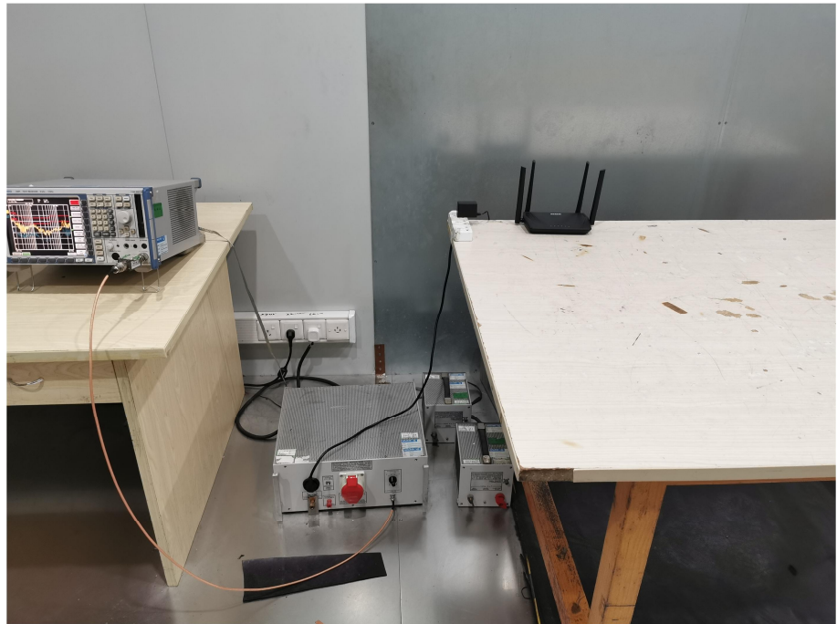
Conducted Emission Test Setup
