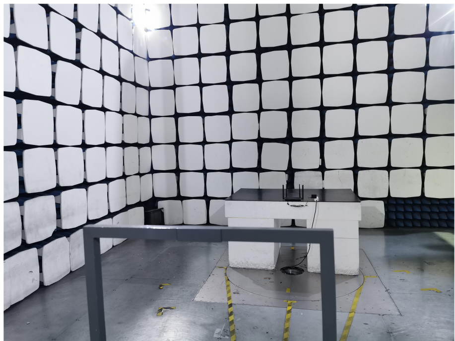
Radiation Emission Test Setup (Below 30MHz)
