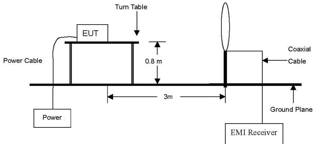
The diagram below shows the test setup that is utilized to make the measurements for emission from 30 MHz to 1 GHz Emissions.
