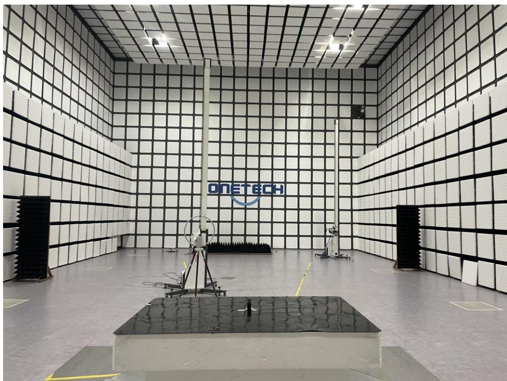
**- Radiated Emission Test (30 MHz ~ 1 GHz)**
