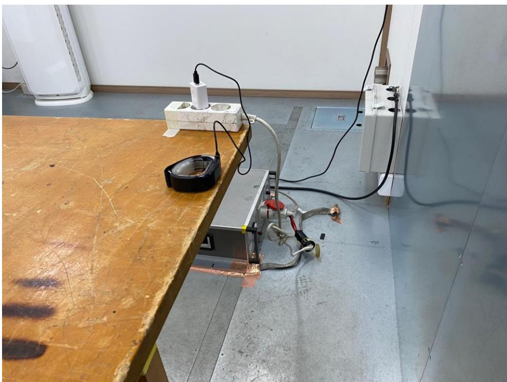
**- Radiated Emission Test (9 kHz ~ 30 MHz)**
