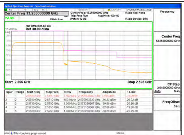
B7 / 15MHz / High CH / QPSK / FULL RB
