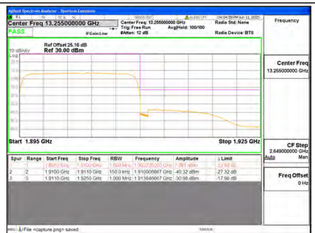
B2 / 15MHz / High CH / QPSK / FULL RB
