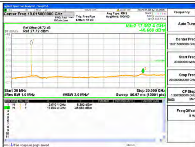
B38-30M-20G / 10MHz / High CH / QPSK
