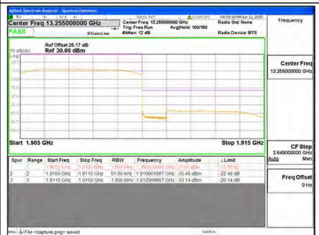
B2 / 5MHz / High CH / QPSK / FULL RB
