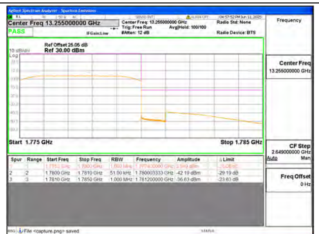
B66 / 5MHz / High CH / QPSK / FULL RB
