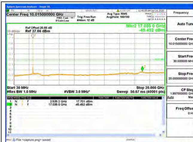
B41-30M-20G / 10MHz / Low CH / QPSK
