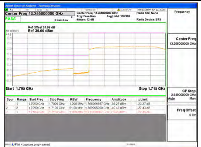
B66 / 5MHz / Low CH / QPSK / FULL RB
