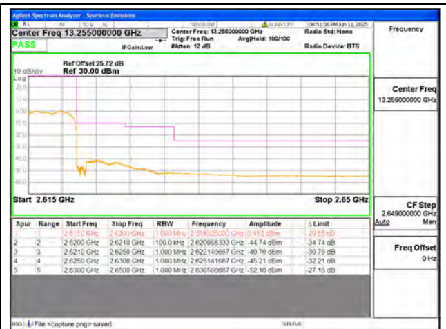
B38 / 10MHz / High CH / QPSK / FULL RB
