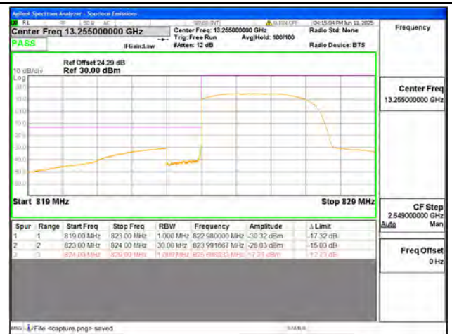
B5 / 3MHz / Low CH / QPSK / FULL RB
