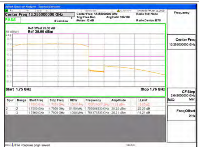
B4 / 5MHz / High CH / QPSK / FULL RB
