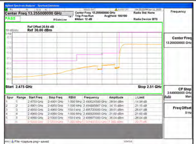
B7 / 15MHz / Low CH / QPSK / FULL RB
