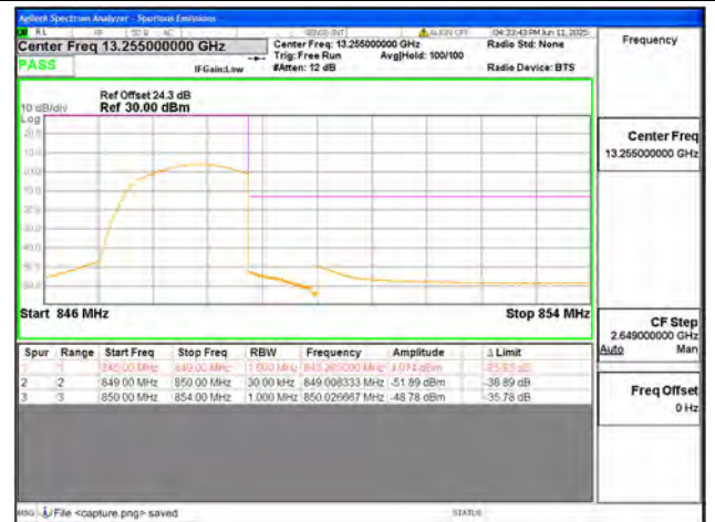
B26 / 1.4MHz / High CH / QPSK / FULL RB
