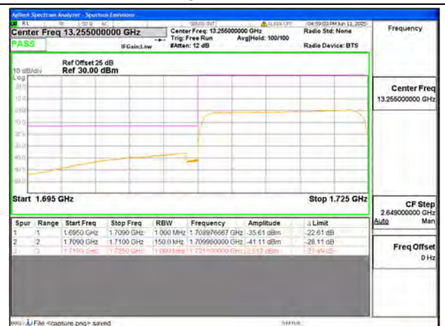
B66 / 15MHz / Low CH / QPSK / FULL RB
