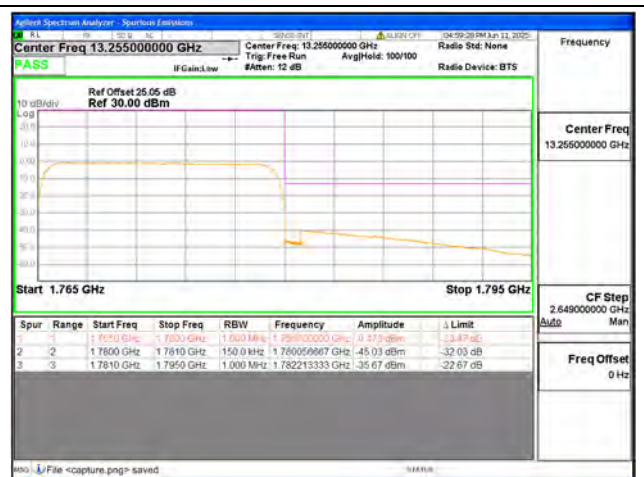
B66 / 15MHz / High CH / QPSK / FULL RB
