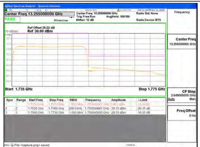
B4 / 20MHz / High CH / QPSK / FULL RB
