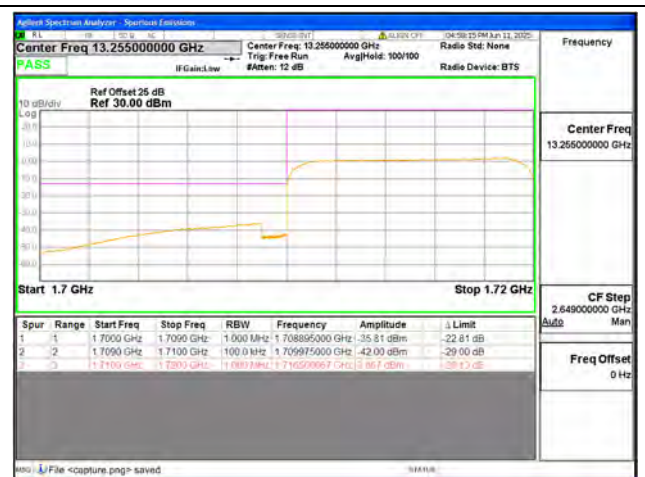
B66 / 10MHz / Low CH / QPSK / FULL RB
