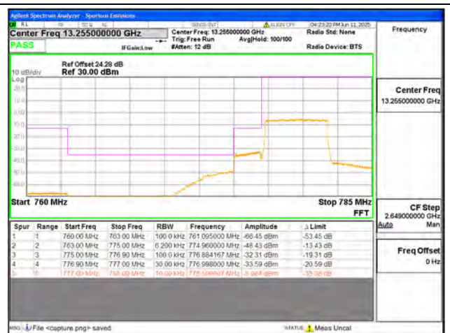
B13 / 5MHz / Low CH / QPSK / FULL RB
