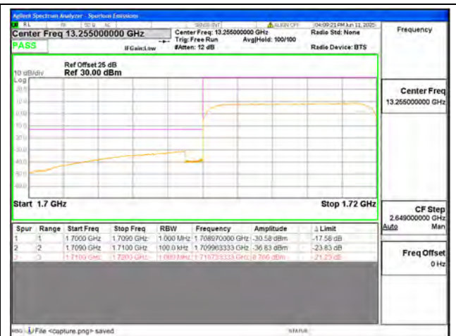
B4 / 10MHz / Low CH / QPSK / FULL RB
