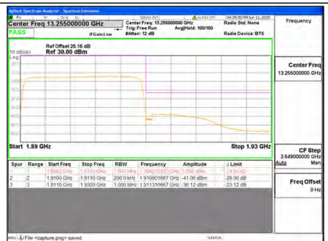
B2 / 20MHz / High CH / QPSK / FULL RB
