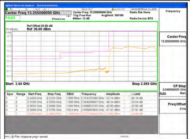
B38 / 15MHz / Low CH / QPSK / FULL RB
