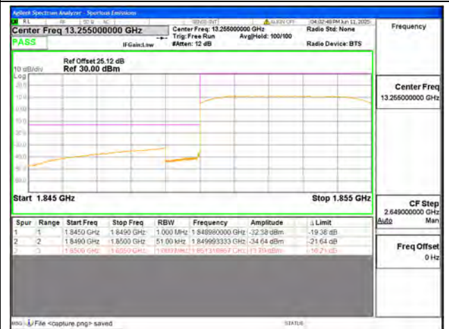
B2 / 5MHz / Low CH / QPSK / FULL RB
