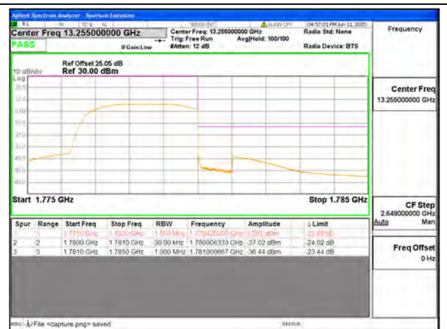
B66 / 3MHz / High CH / QPSK / FULL RB
