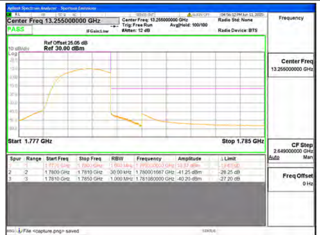
B66 / 1.4MHz / High CH / QPSK / FULL RB
