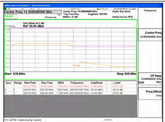
B26 / 10MHz / High CH / QPSK / FULL RB
