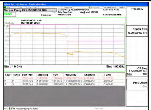
B2 / 10MHz / High CH / QPSK / FULL RB
