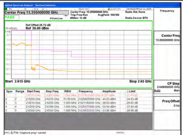
B38 / 5MHz / High CH / QPSK / FULL RB
