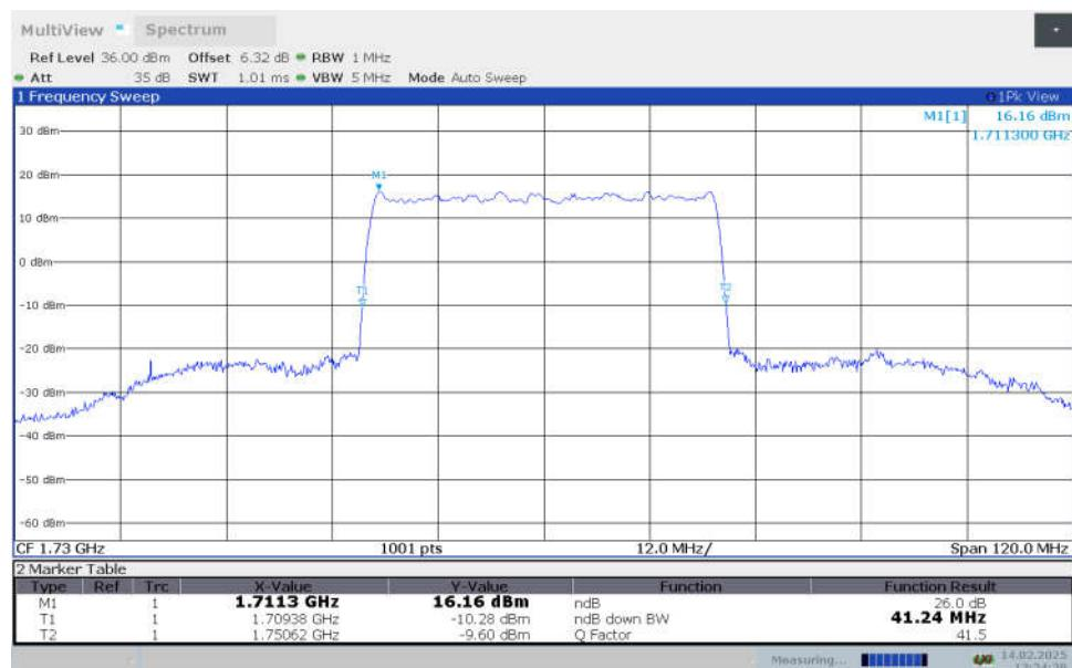
**n66,40MHz Bandwidth,DFT-s-256QAM (-26dBc OBW)**
