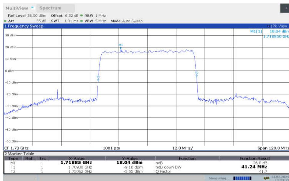
**n66,40MHz Bandwidth,DFT-s-16QAM (-26dBc OBW)**
