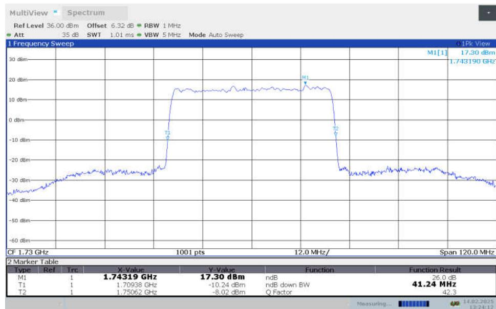
**n66,40MHz Bandwidth,DFT-s-64QAM (-26dBc OBW)**
