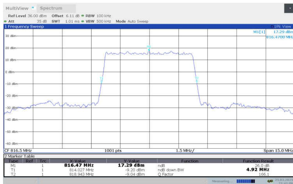
**n26(814MHz-824MHz),5MHz Bandwidth,DFT-s-QPSK (-26dBc OBW)**
