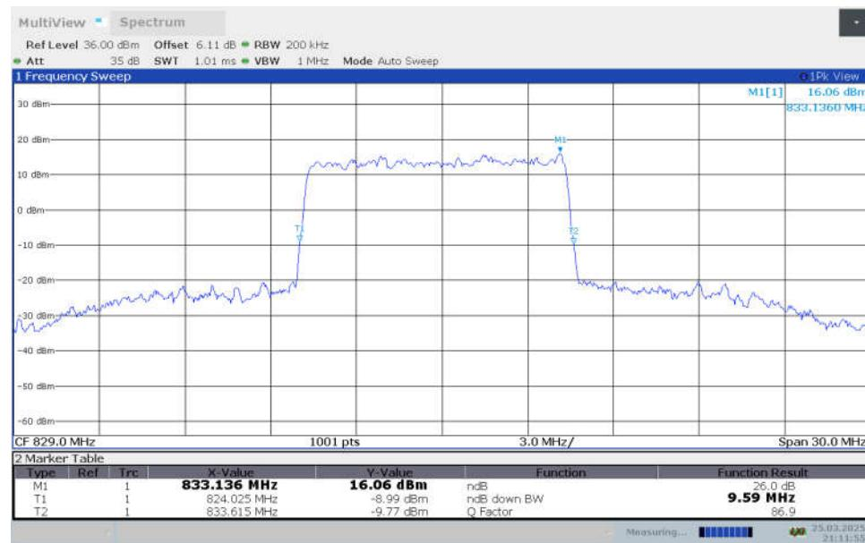
**n26(824MHz-849MHz),10MHz Bandwidth,DFT-s-256QAM (-26dBc OBW)**
