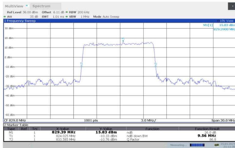
**n26(824MHz-849MHz),10MHz Bandwidth,DFT-s-64QAM (-26dBc OBW)**
