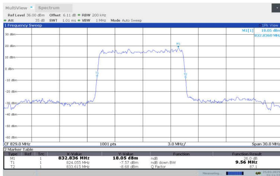
**n26(824MHz-849MHz),10MHz Bandwidth,DFT-s-16QAM (-26dBc OBW)**
