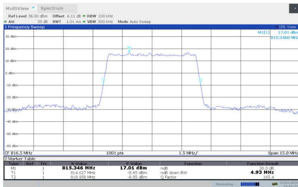
**n26(814MHz-824MHz),5MHz Bandwidth,DFT-s-16QAM (-26dBc OBW)**
