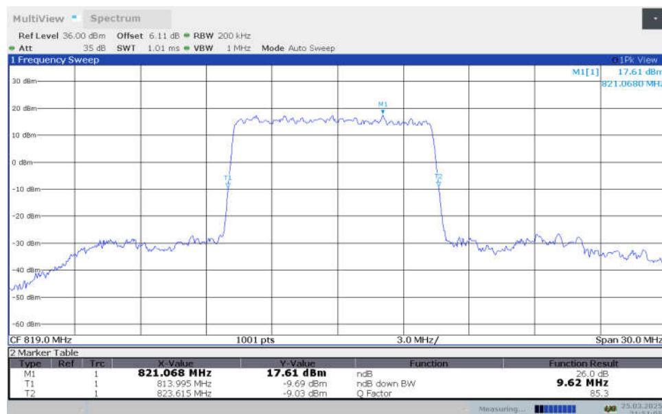
**n26(814MHz-824MHz),10MHz Bandwidth,DFT-s-QPSK (-26dBc OBW)**
