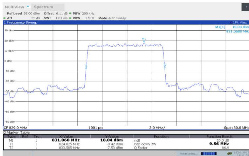
**n26(824MHz-849MHz),10MHz Bandwidth,DFT-s-QPSK (-26dBc OBW)**
