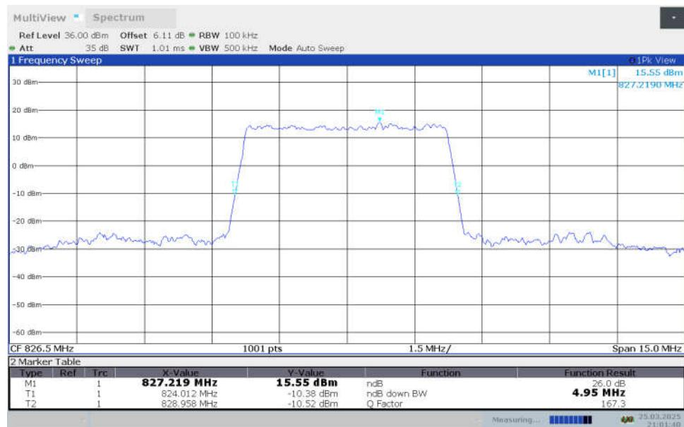
**n26(824MHz-849MHz),5MHz Bandwidth,DFT-s-64QAM (-26dBc OBW)**
