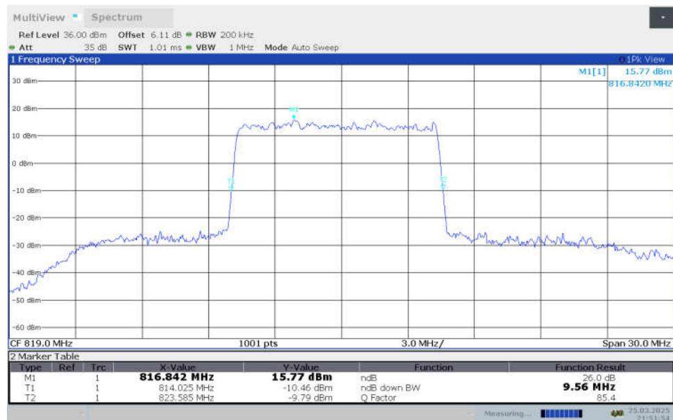
**n26(814MHz-824MHz),10MHz Bandwidth,DFT-s-256QAM (-26dBc OBW)**
