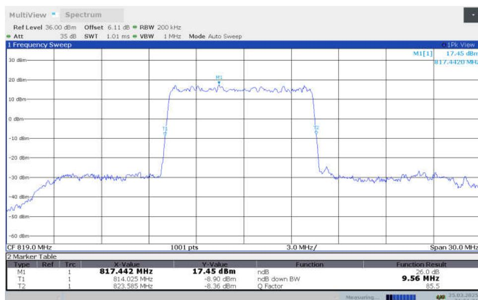
**n26(814MHz-824MHz),10MHz Bandwidth,DFT-s-16QAM (-26dBc OBW)**
