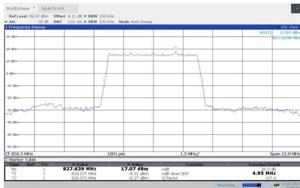
**n26(824MHz-849MHz),5MHz Bandwidth,DFT-s-QPSK (-26dBc OBW)**
