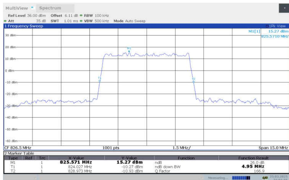
**n26(824MHz-849MHz),5MHz Bandwidth,DFT-s-256QAM (-26dBc OBW)**
