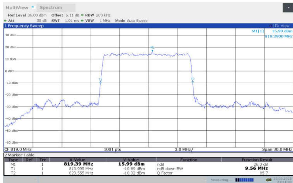
**n26(814MHz-824MHz),10MHz Bandwidth,DFT-s-64QAM (-26dBc OBW)**
