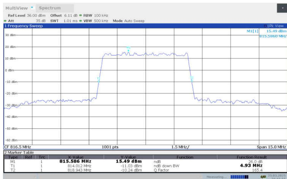
**n26(814MHz-824MHz),5MHz Bandwidth,DFT-s-256QAM (-26dBc OBW)**
