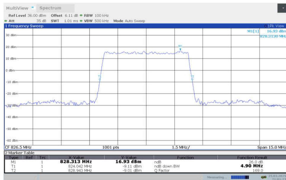
**n26(824MHz-849MHz),5MHz Bandwidth,DFT-s-16QAM (-26dBc OBW)**
