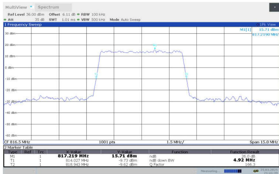
**n26(814MHz-824MHz),5MHz Bandwidth,DFT-s-64QAM (-26dBc OBW)**
