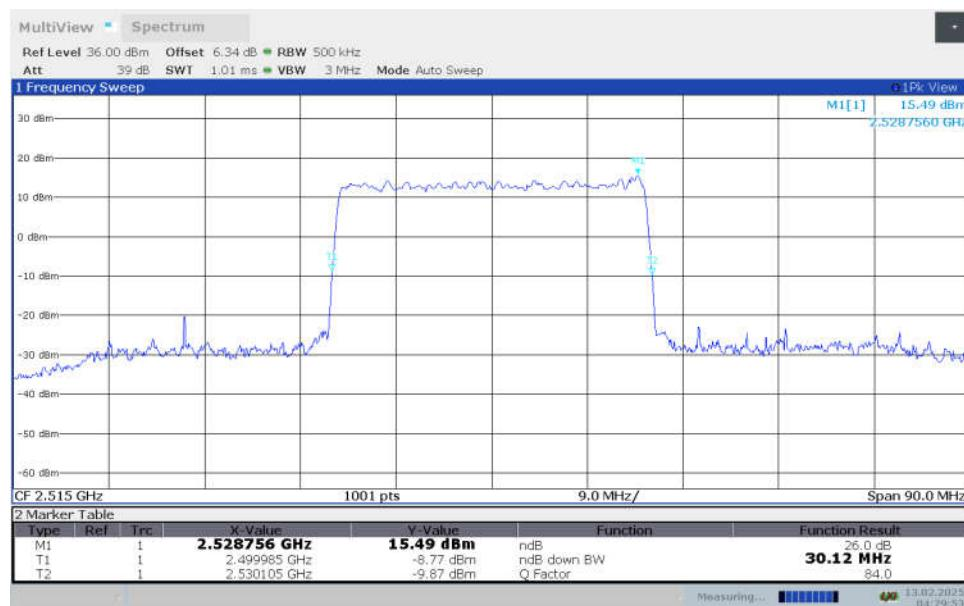
**n7,30MHz Bandwidth,DFT-s-16QAM (-26dBc OBW)**
