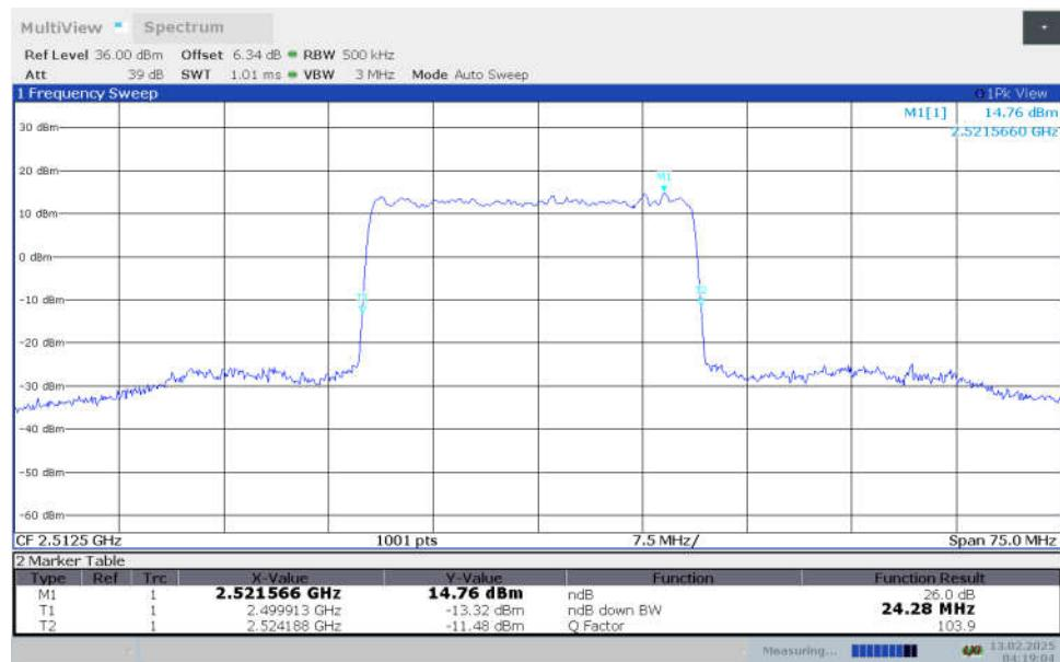
**n7,25MHz Bandwidth,DFT-s-64QAM (-26dBc OBW)**
