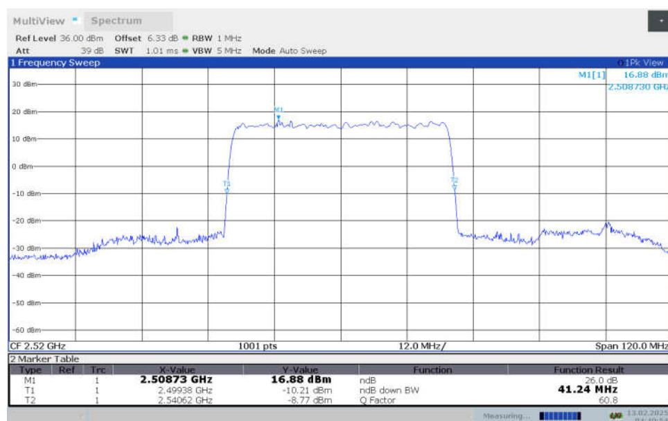
**n7,40MHz Bandwidth,DFT-s-16QAM (-26dBc OBW)**
