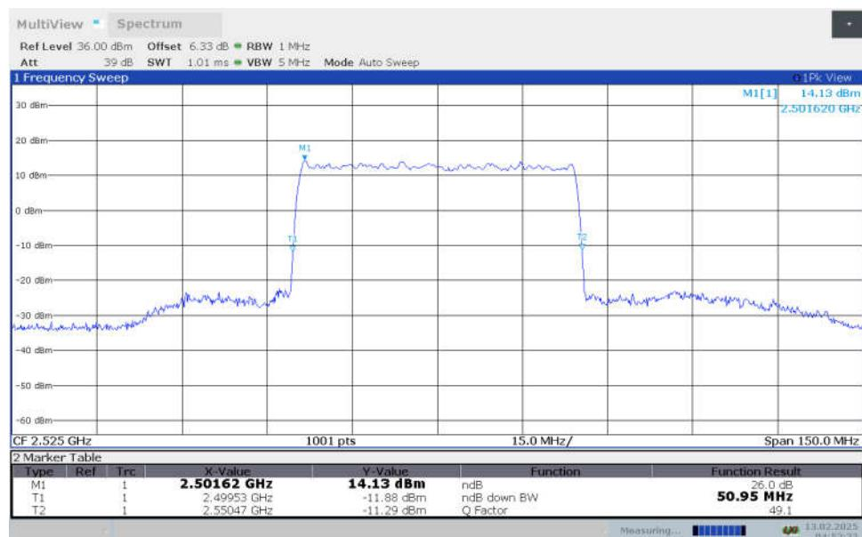
**n7,50MHz Bandwidth,DFT-s-256QAM (-26dBc OBW)**
