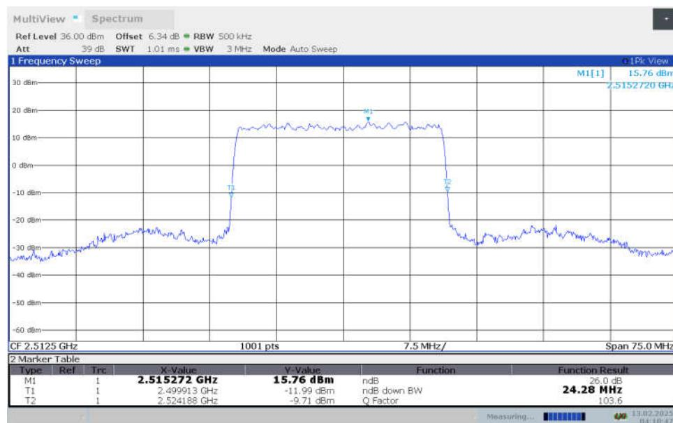
**n7,25MHz Bandwidth,DFT-s-16QAM (-26dBc OBW)**
