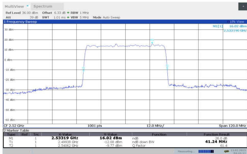
**n7,40MHz Bandwidth,DFT-s-64QAM (-26dBc OBW)**
