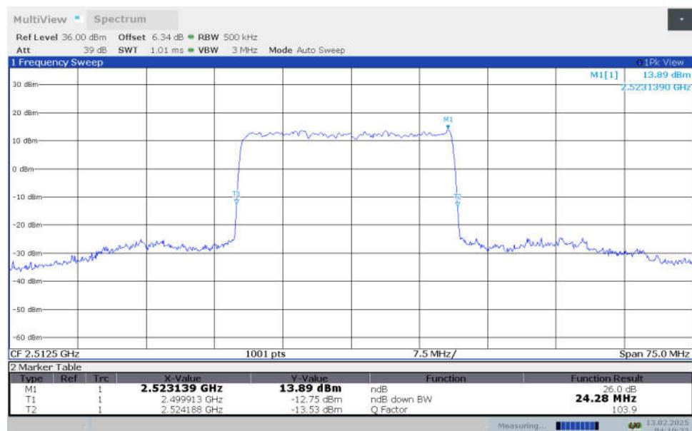
**n7,25MHz Bandwidth,DFT-s-256QAM (-26dBc OBW)**
