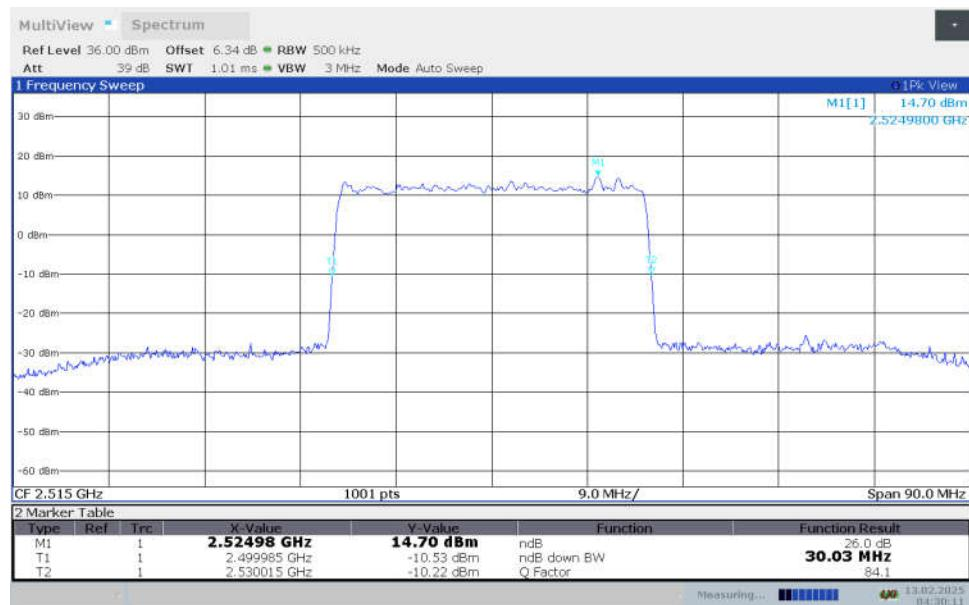
**n7,30MHz Bandwidth,DFT-s-64QAM (-26dBc OBW)**
