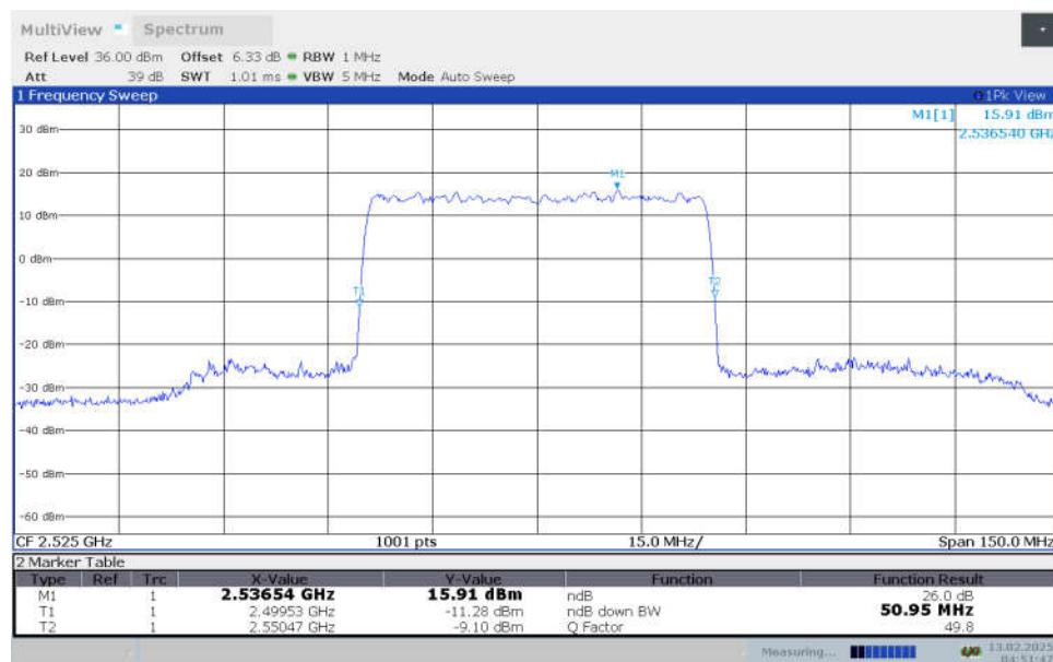
**n7,50MHz Bandwidth,DFT-s-16QAM (-26dBc OBW)**
