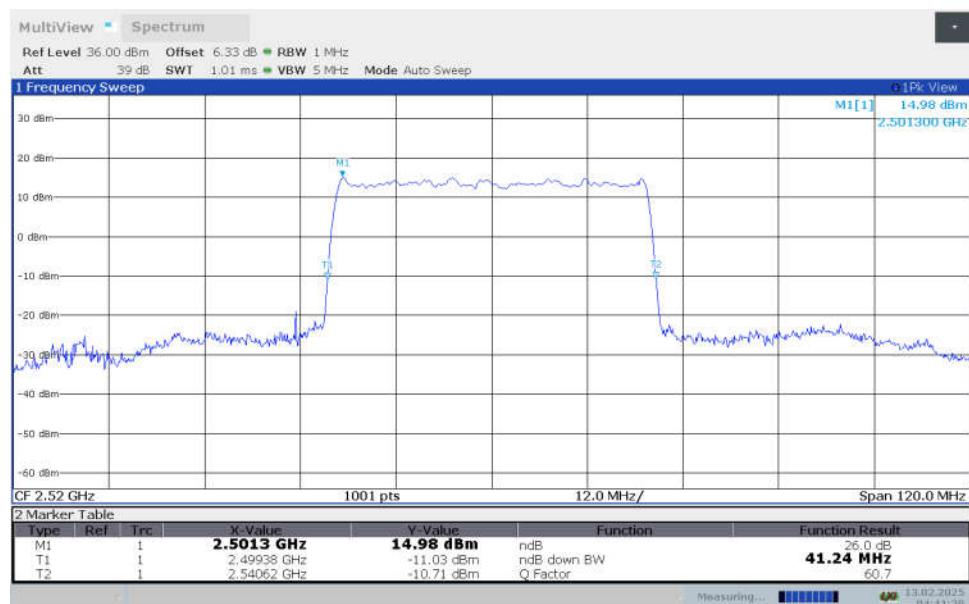
**n7,40MHz Bandwidth,DFT-s-256QAM (-26dBc OBW)**
