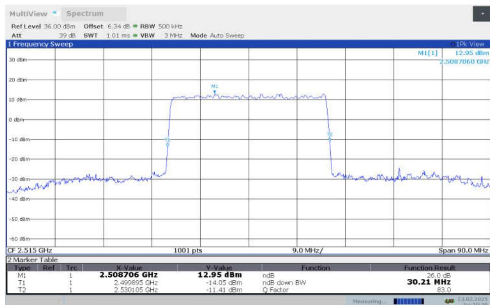
**n7,30MHz Bandwidth,DFT-s-256QAM (-26dBc OBW)**
