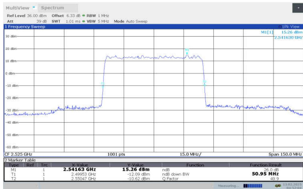
**n7,50MHz Bandwidth,DFT-s-64QAM (-26dBc OBW)**
