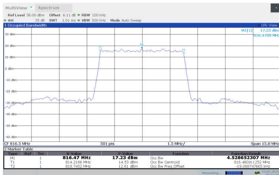
**n26(814MHz-824MHz),5MHz Bandwidth,DFT-s-QPSK (99% OBW)**
