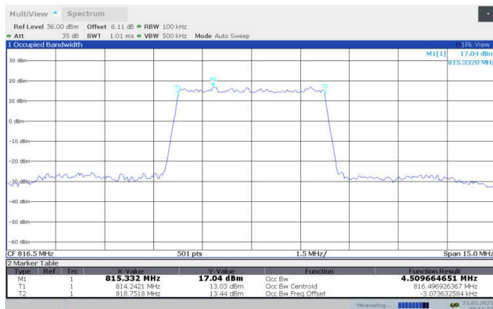
**n26(814MHz-824MHz),5MHz Bandwidth,DFT-s-16QAM (99% OBW)**
