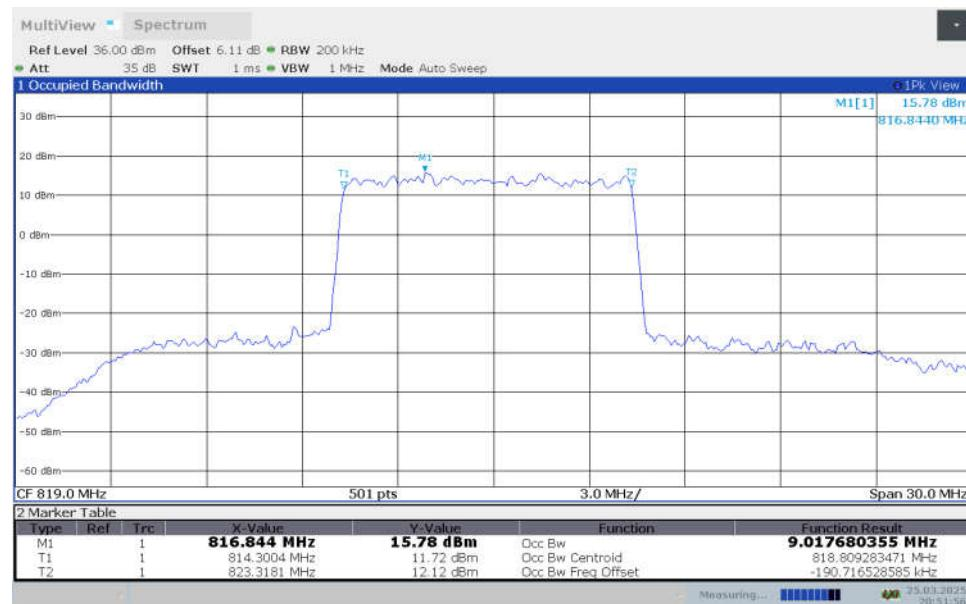
**n26(814MHz-824MHz),10MHz Bandwidth,DFT-s-256QAM (99% OBW)**
