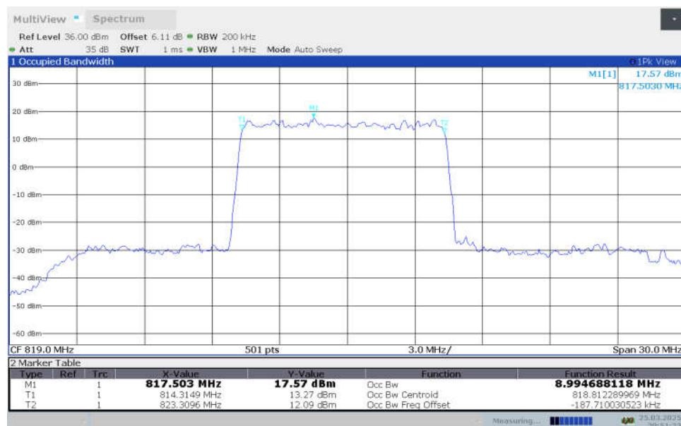
**n26(814MHz-824MHz),10MHz Bandwidth,DFT-s-16QAM (99% OBW)**
