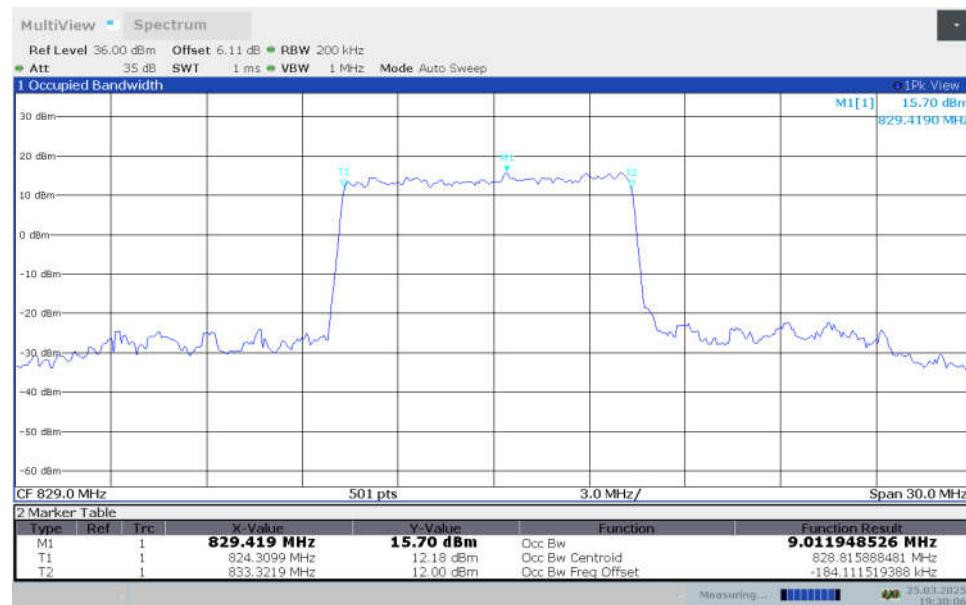
**n26(824MHz-849MHz),10MHz Bandwidth,DFT-s-64QAM (99% OBW)**
