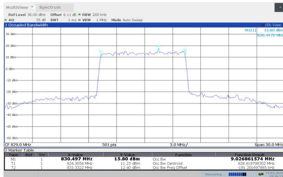
**n26(824MHz-849MHz),10MHz Bandwidth,DFT-s-256QAM (99% OBW)**
