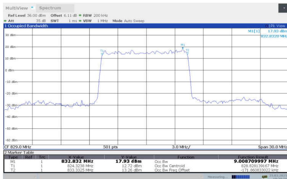
**n26(824MHz-849MHz),10MHz Bandwidth,DFT-s-16QAM (99% OBW)**
