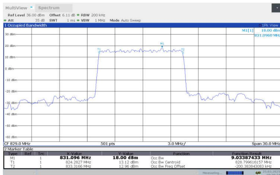
**n26(824MHz-849MHz),10MHz Bandwidth,DFT-s-QPSK (99% OBW)**
