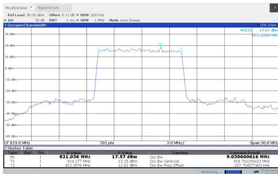
**n26(814MHz-824MHz),10MHz Bandwidth,DFT-s-QPSK (99% OBW)**
