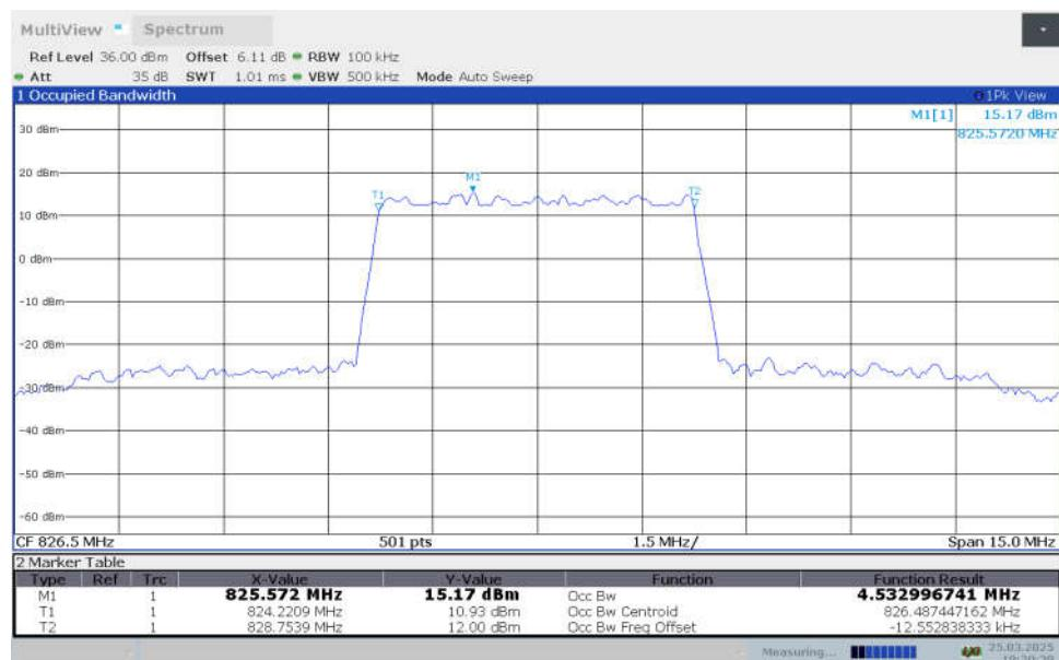
**n26(824MHz-849MHz),5MHz Bandwidth,DFT-s-256QAM (99% OBW)**
