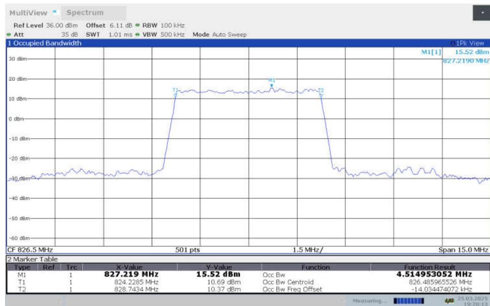
**n26(824MHz-849MHz),5MHz Bandwidth,DFT-s-64QAM (99% OBW)**
