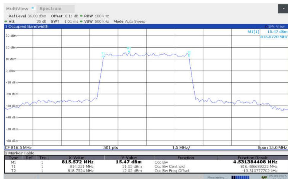
**n26(814MHz-824MHz),5MHz Bandwidth,DFT-s-256QAM (99% OBW)**
