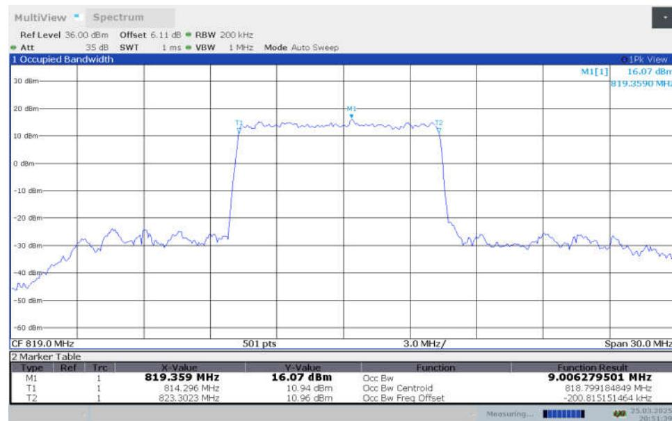
**n26(814MHz-824MHz),10MHz Bandwidth,DFT-s-64QAM (99% OBW)**
