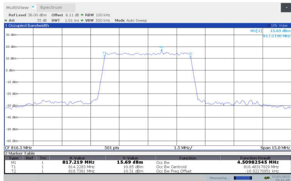
**n26(814MHz-824MHz),5MHz Bandwidth,DFT-s-64QAM (99% OBW)**
