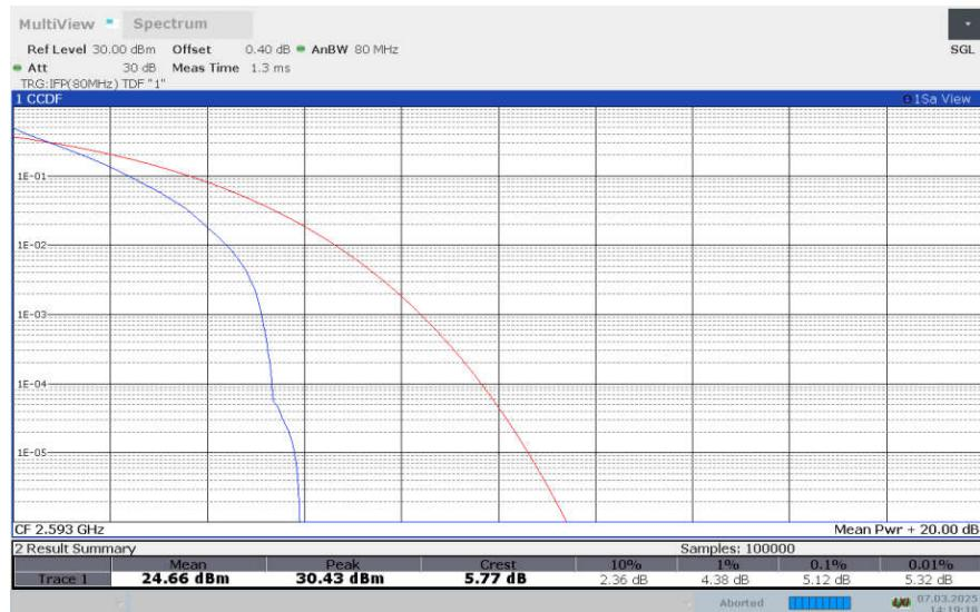
**LTE Band 41, 20MHz Bandwidth, 16QAM**
