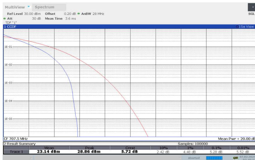
**LTE Band 12, 10MHz Bandwidth, 16QAM**
