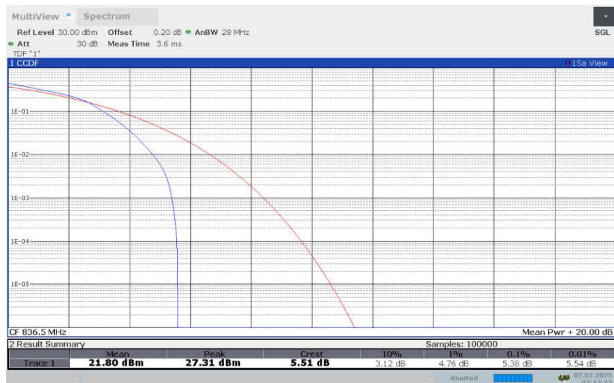
**LTE Band 26 , 1.4MHz Bandwidth,64QAM**
