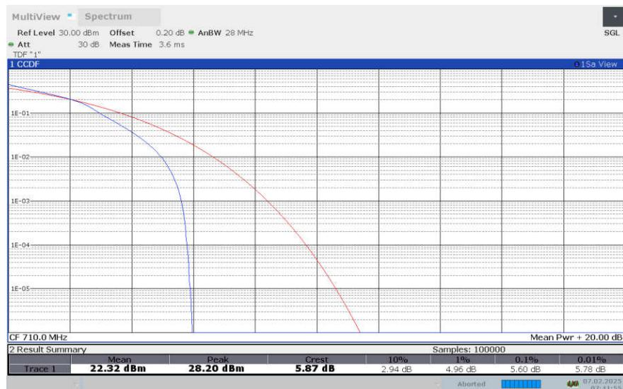
**LTE Band 17, 5MHz Bandwidth, 64QAM**
