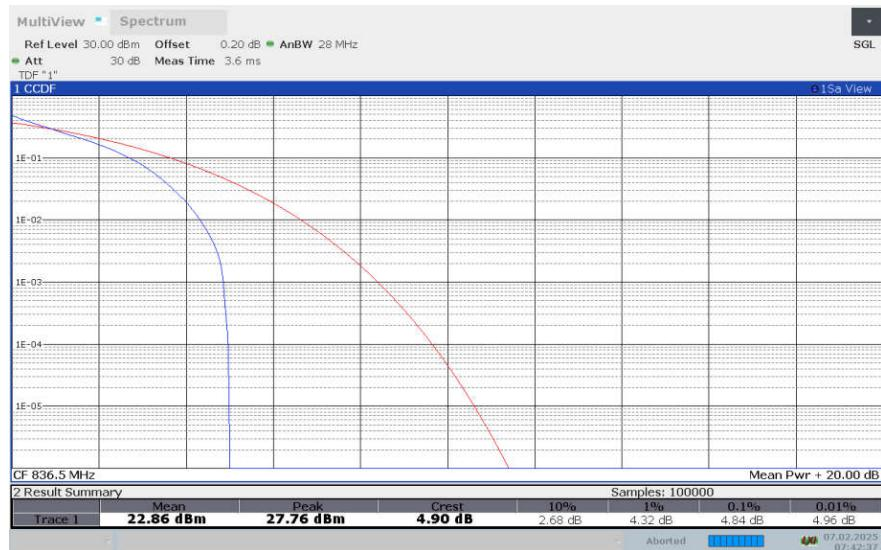
**LTE Band 26 , 1.4MHz Bandwidth,16QAM**
