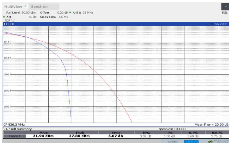
**LTE Band 26 , 3MHz Bandwidth,64QAM**
