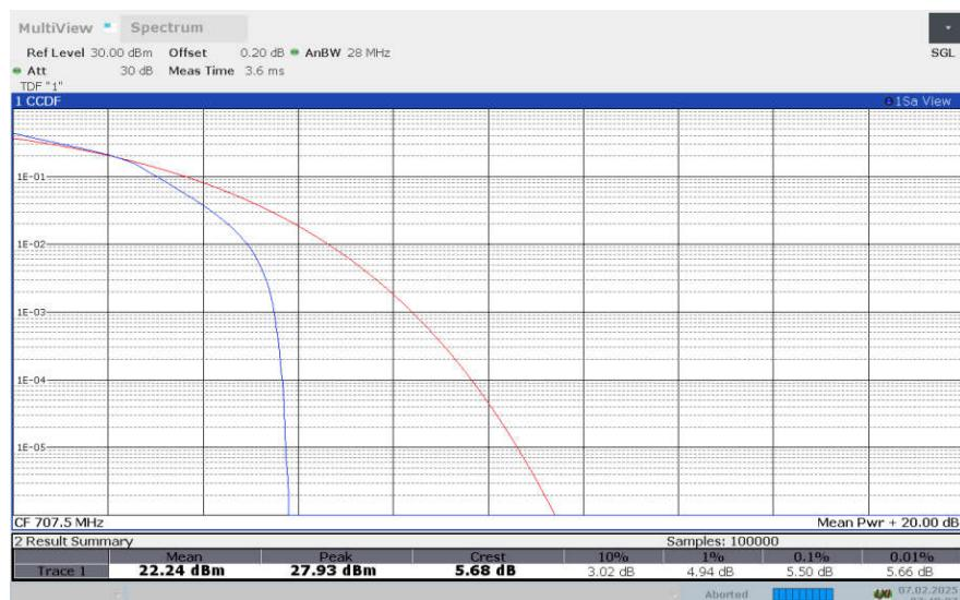
**LTE Band 12 , 3MHz Bandwidth,64QAM**
