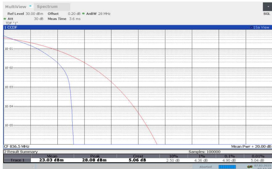
**LTE Band 26 , 5MHz Bandwidth,16QAM**
