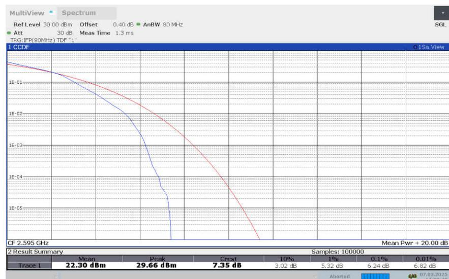
**LTE Band 38, 15MHz Bandwidth, 64QAM**
