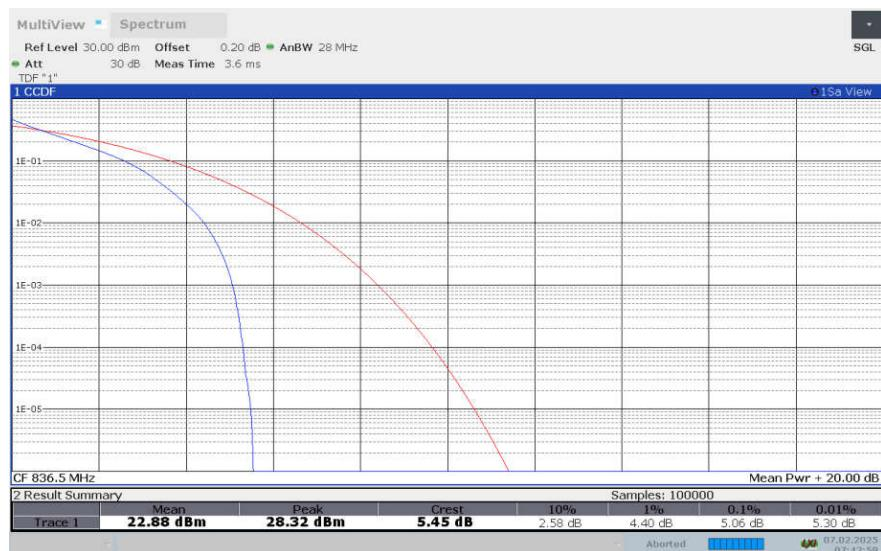
**LTE Band 26 , 3MHz Bandwidth,16QAM**
