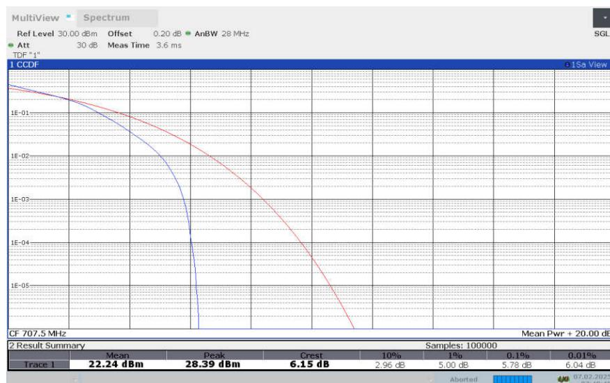
**LTE Band 12, 10MHz Bandwidth, 64QAM**
