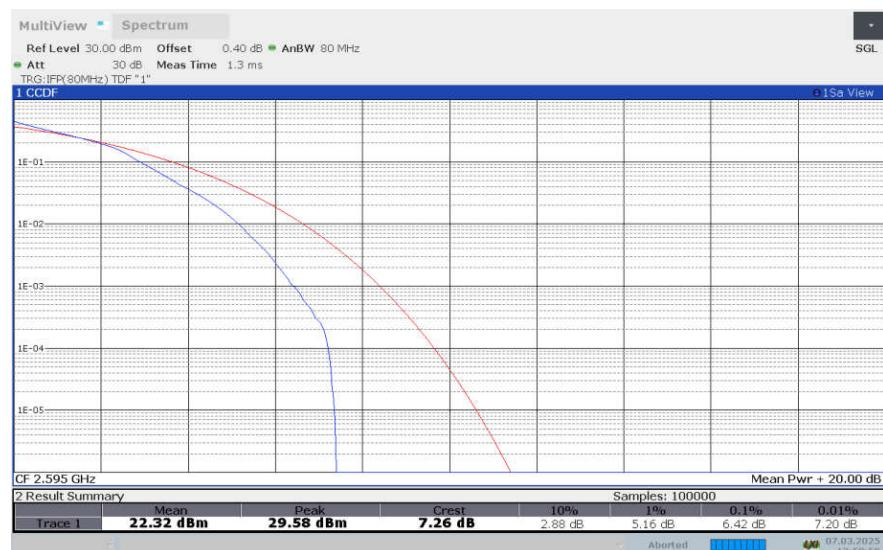
**LTE Band 38, 10MHz Bandwidth, 64QAM**
