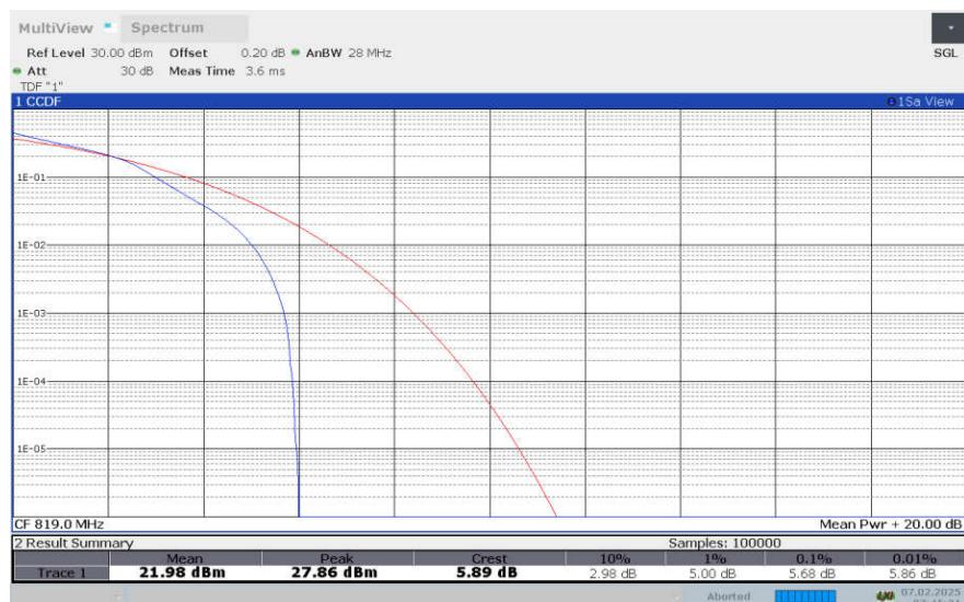
**LTE Band 26 , 5MHz Bandwidth,64QAM**
