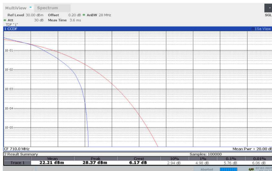
**LTE Band 17, 10MHz Bandwidth, 64QAM**
