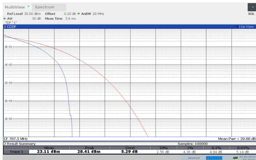
**LTE Band 12 , 3MHz Bandwidth,16QAM**
