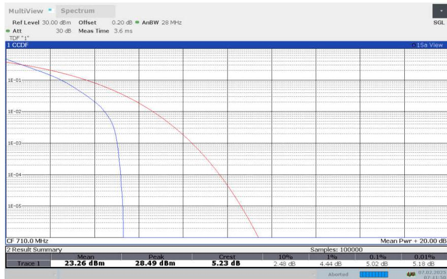
**LTE Band 17, 5MHz Bandwidth, 16QAM**
