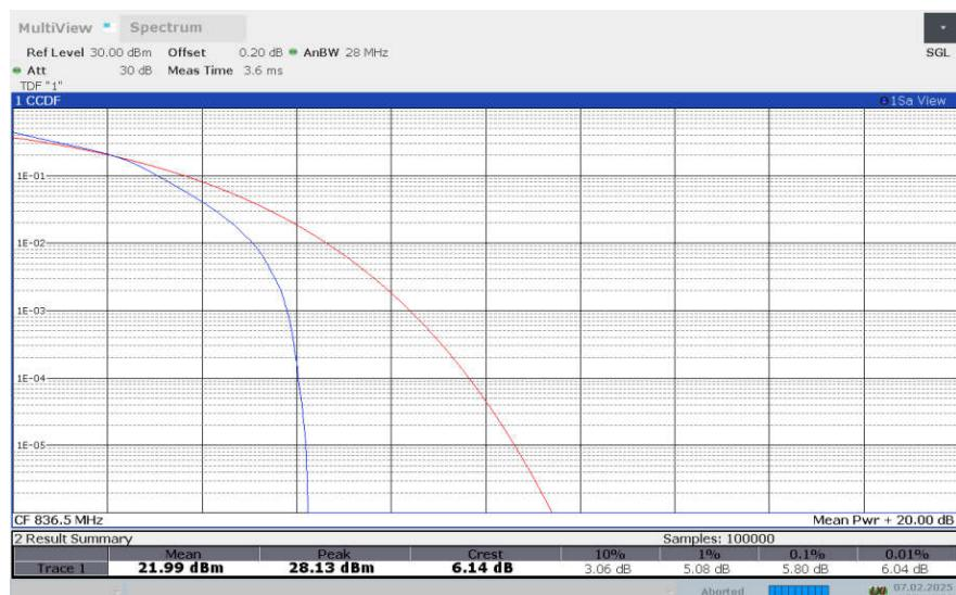
**LTE Band 26 , 15MHz Bandwidth,64QAM**
