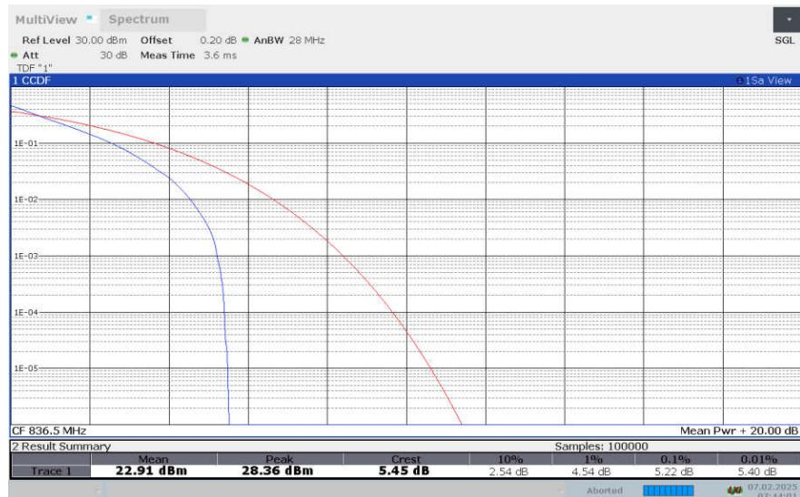
**LTE Band 26 , 15MHz Bandwidth,16QAM**
