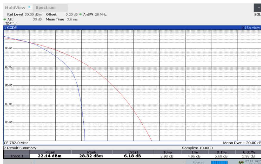
**LTE Band 13, 10MHz Bandwidth, 64QAM**
