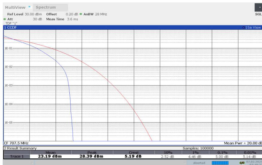
**LTE Band 12 , 5MHz Bandwidth,16QAM**
