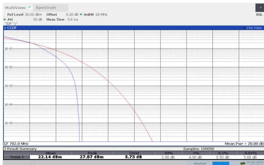
**LTE Band 13, 5MHz Bandwidth, 64QAM**
