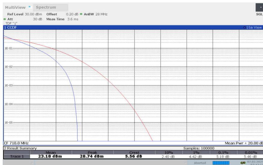
**LTE Band 17, 10MHz Bandwidth, 16QAM**
