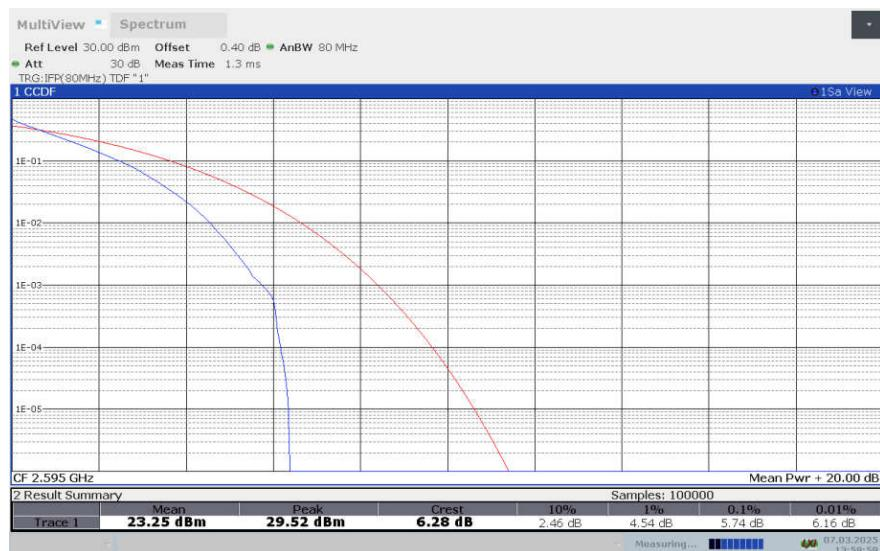
**LTE Band 38, 5MHz Bandwidth, 16QAM**
