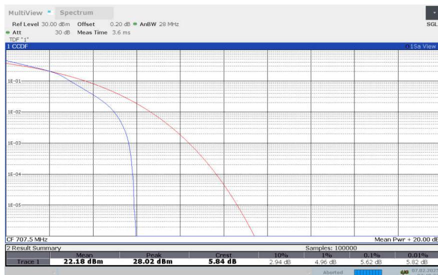
**LTE Band 12 , 5MHz Bandwidth,64QAM**
