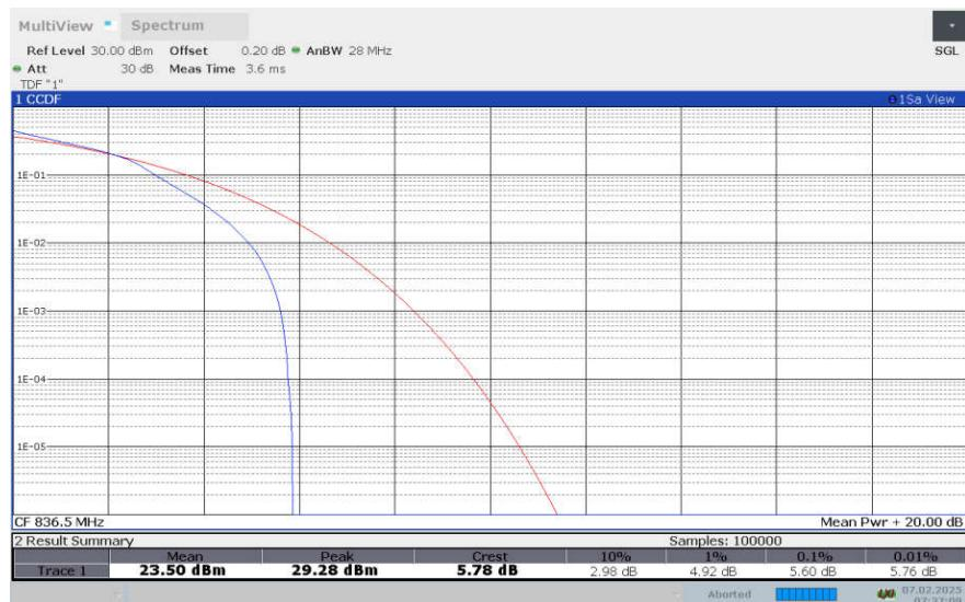
**LTE Band 5, 5MHz Bandwidth, 64QAM**
