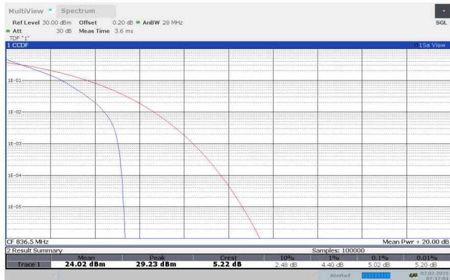
**LTE Band 5, 5MHz Bandwidth, 16QAM**
