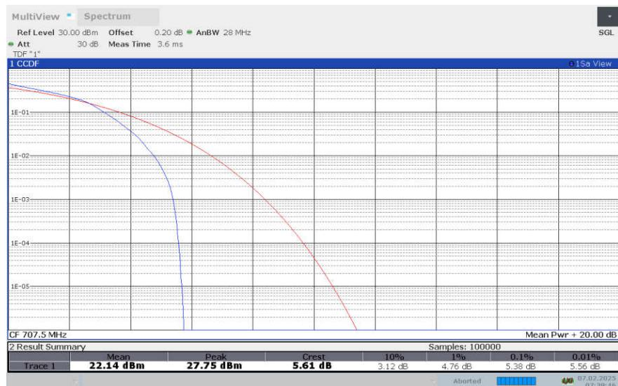
**LTE Band 12 , 1.4MHz Bandwidth,64QAM**
