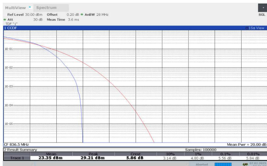
**LTE Band 5 , 1.4MHz Bandwidth,64QAM**
