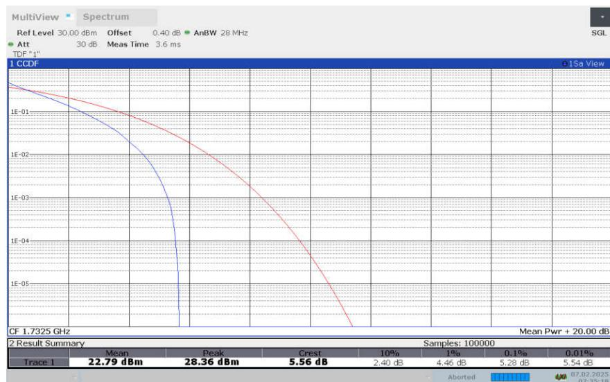
**LTE Band 4, 10MHz Bandwidth, 16QAM**
