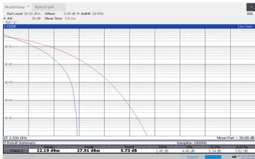
**LTE Band 7, 10MHz Bandwidth, 16QAM**
