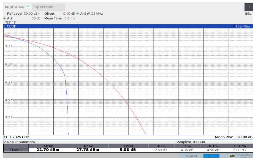
**LTE Band 4 , 1.4MHz Bandwidth,16QAM**
