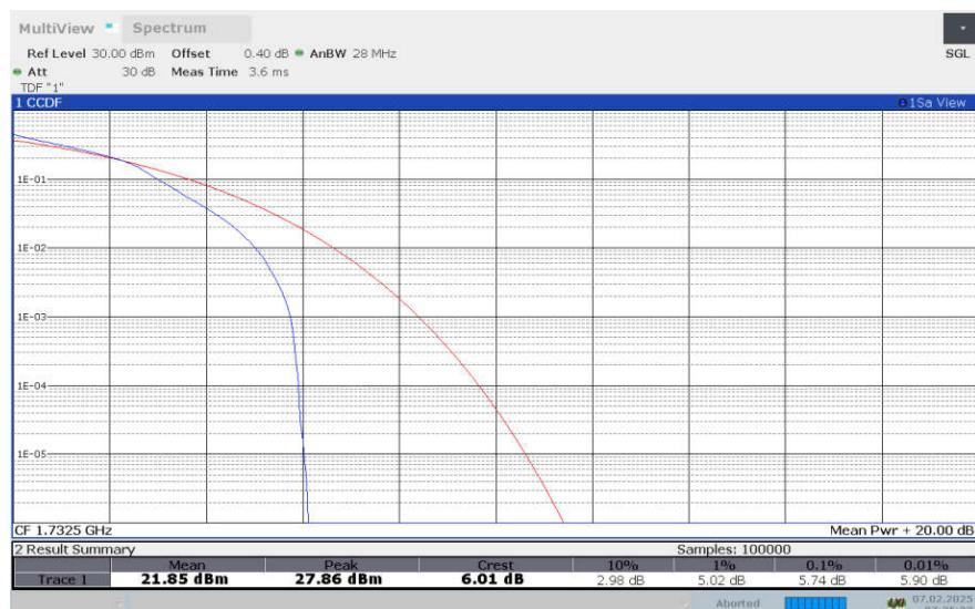
**LTE Band 4, 5MHz Bandwidth, 64QAM**
