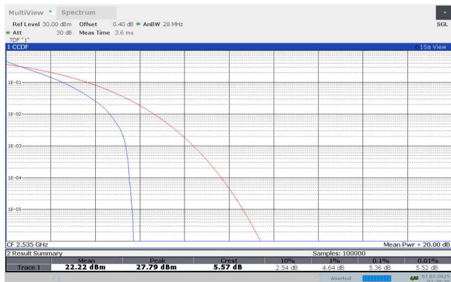
**LTE Band 7, 15MHz Bandwidth, 16QAM**
