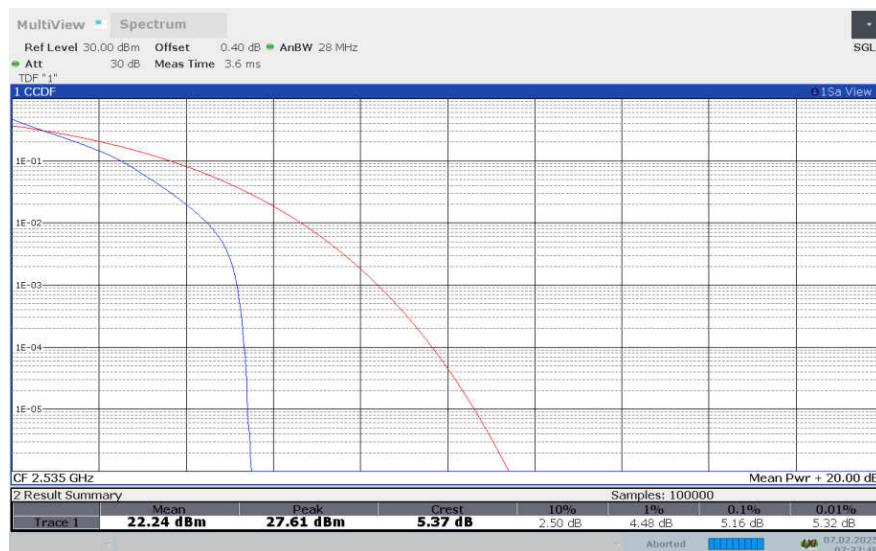
**LTE Band 7, 5MHz Bandwidth, 16QAM**
