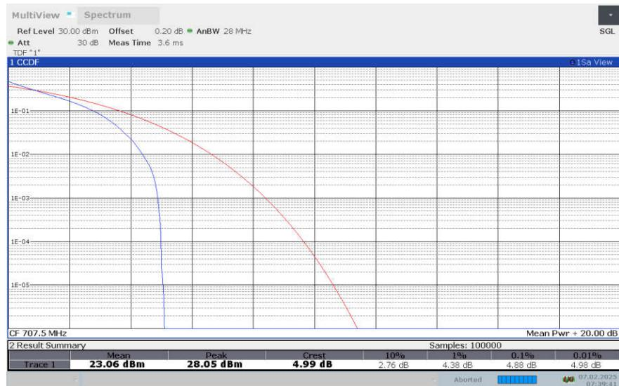
**LTE Band 12 , 1.4MHz Bandwidth,16QAM**
