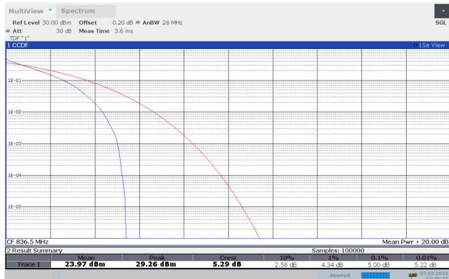
**LTE Band 5 , 3MHz Bandwidth,16QAM**
