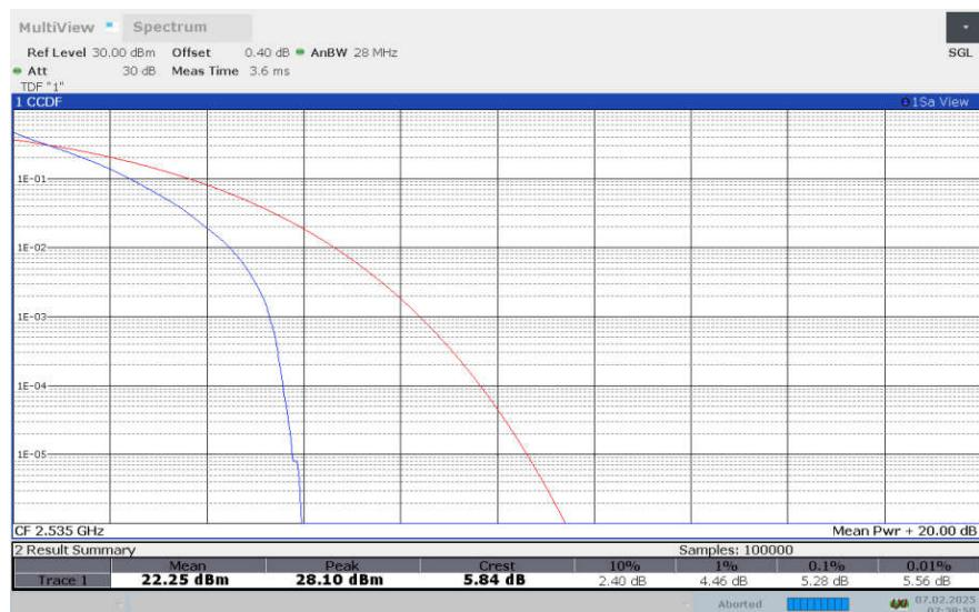
**LTE Band 7, 20MHz Bandwidth, 16QAM**
