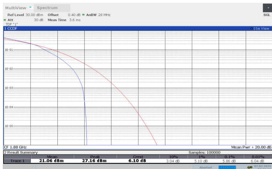
**LTE Band 2 , 15MHz Bandwidth,64QAM**
