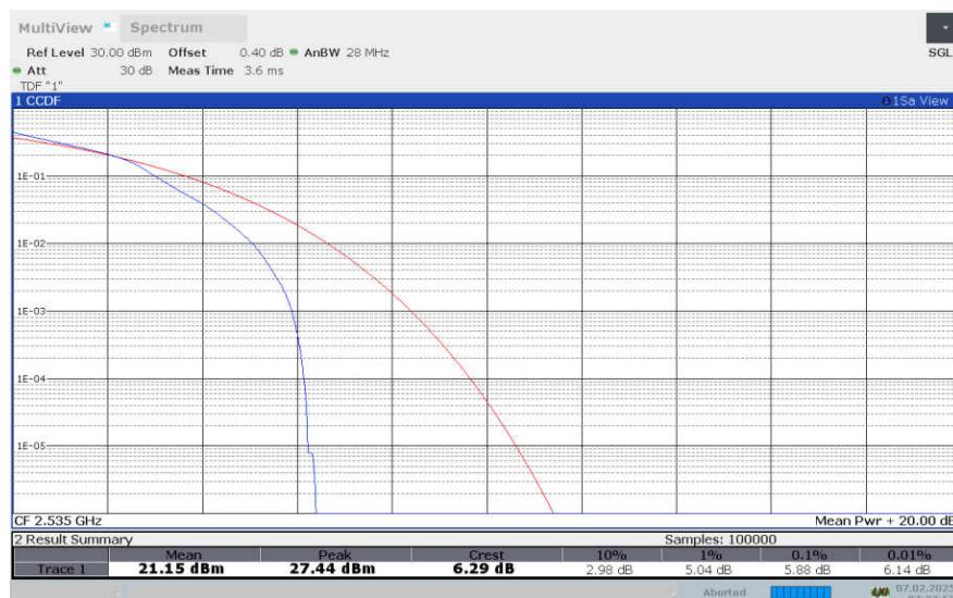
**LTE Band 7, 5MHz Bandwidth, 64QAM**
