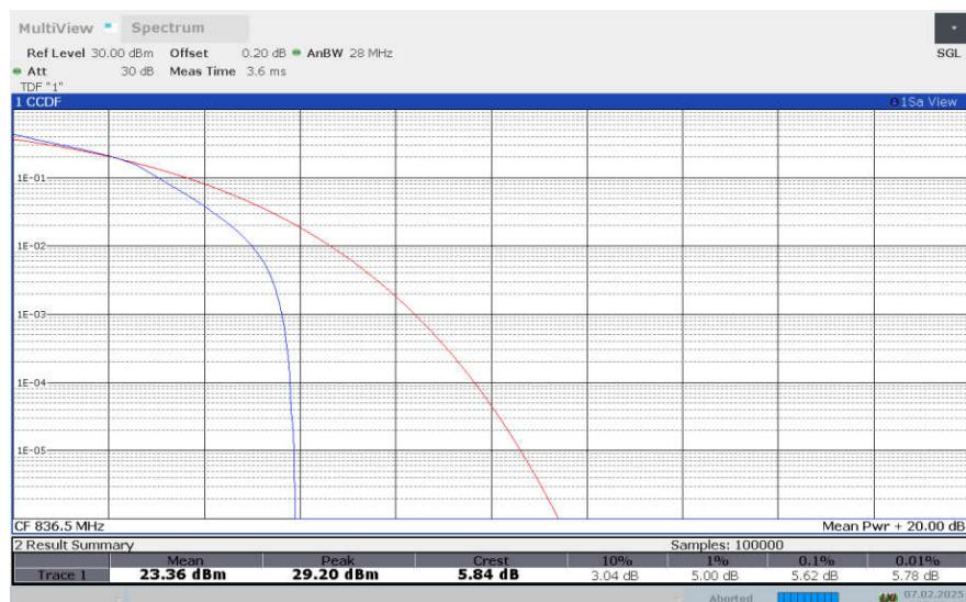
**LTE Band 5 , 3MHz Bandwidth,64QAM**
