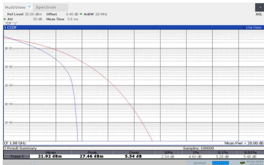
**LTE Band 2, 15MHz Bandwidth, 16QAM**
