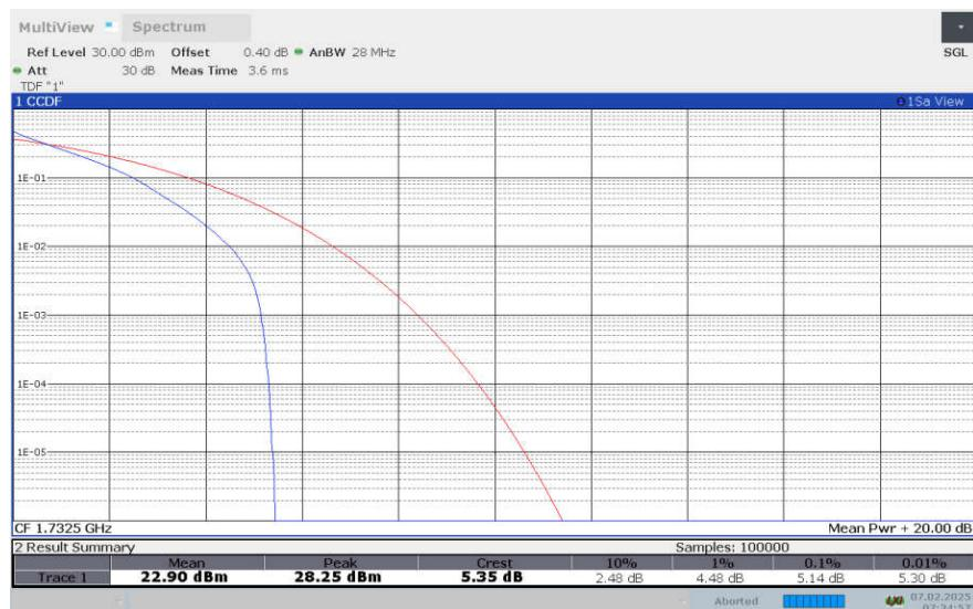
**LTE Band 4, 5MHz Bandwidth, 16QAM**
