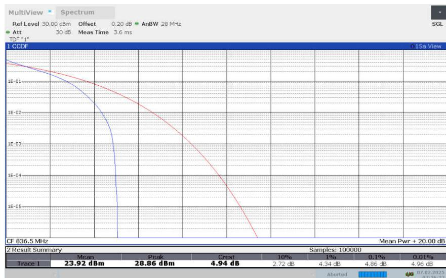
**LTE Band 5 , 1.4MHz Bandwidth,16QAM**
