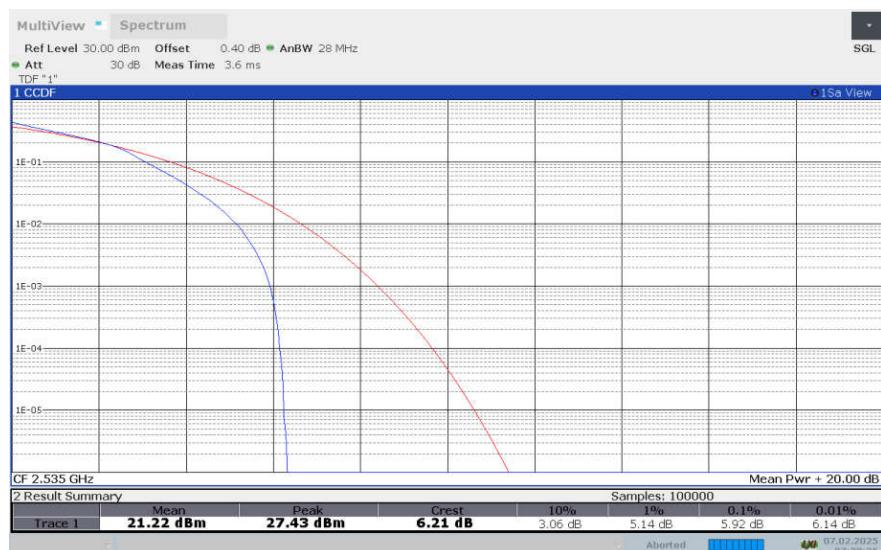
**LTE Band 7, 15MHz Bandwidth, 64QAM**
