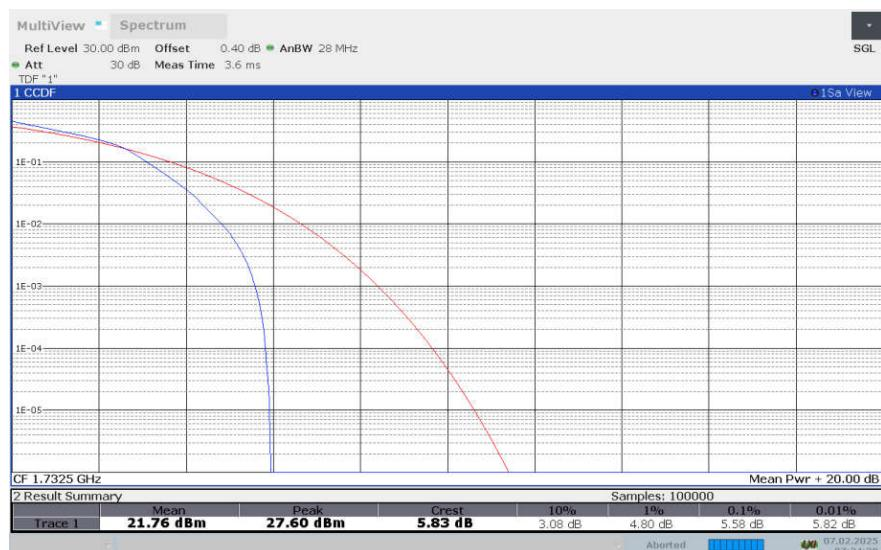
**LTE Band 4 , 1.4MHz Bandwidth,64QAM**
