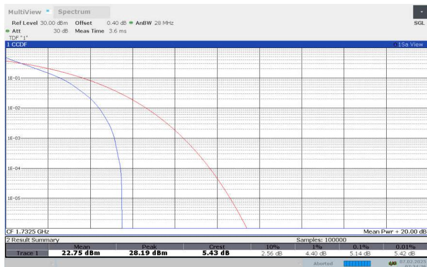
**LTE Band 4 , 3MHz Bandwidth,16QAM**
