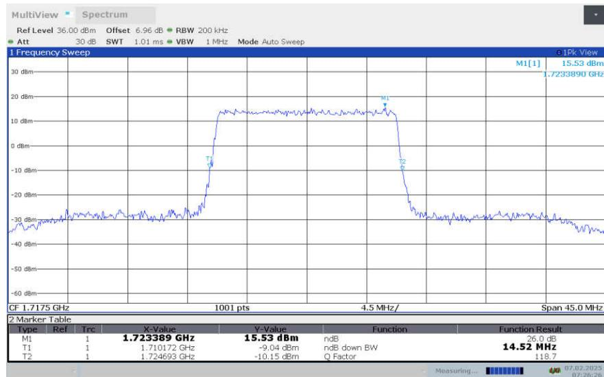
**LTE Band 66 , 15MHz Bandwidth,LOW,16QAM (-26dBc OBW)**
