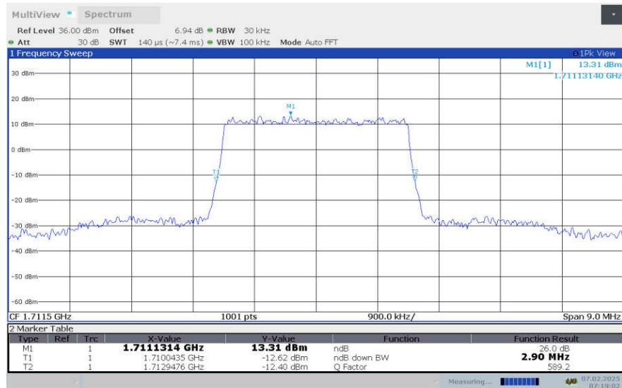
**LTE Band 66, 3MHz Bandwidth,LOW,64QAM (-26dBc OBW)**
