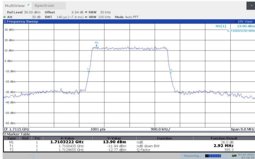
**LTE Band 66, 3MHz Bandwidth,LOW,16QAM (-26dBc OBW)**
