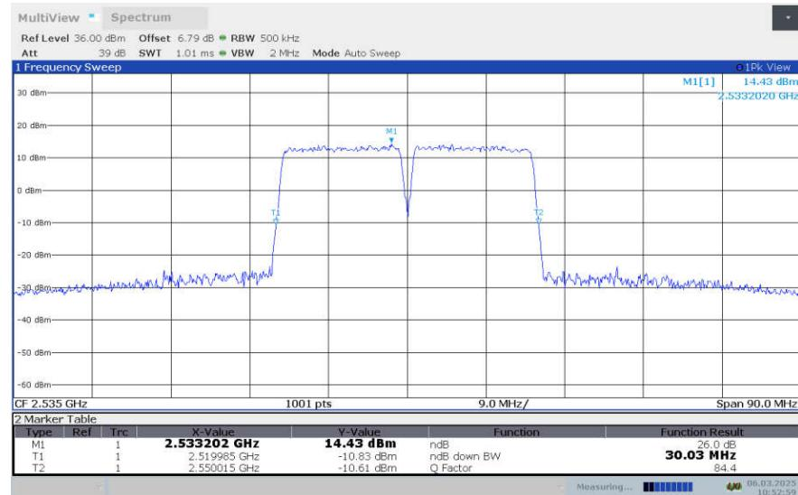
**LTE CA\_7C , 15MHz+15MHz Bandwidth,16QAM (-26dBc OBW)**
