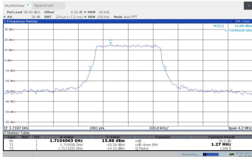
**LTE Band 66 , 1.4MHz Bandwidth,LOW,16QAM (-26dBc OBW)**
