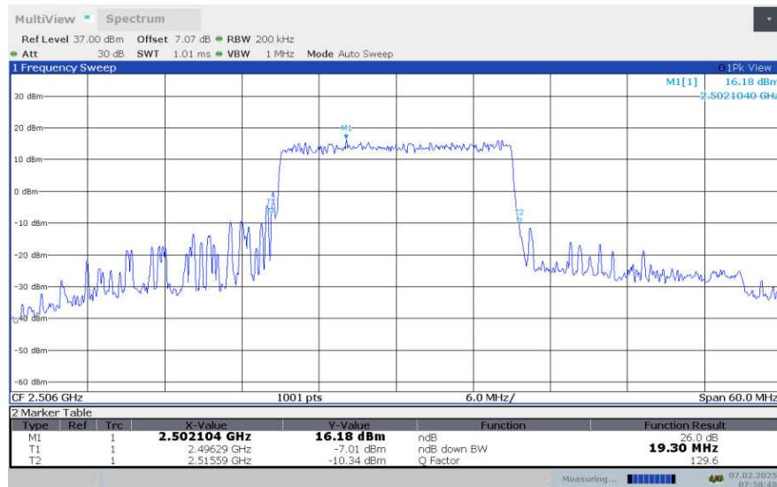
**LTE Band 41 , 20MHz Bandwidth,LOW,16QAM (-26dBc OBW)**
