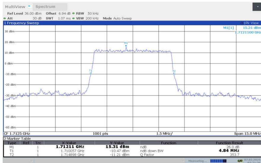
**LTE Band 66 , 5MHz Bandwidth,LOW,64QAM (-26dBc OBW)**
