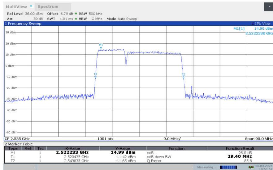
**LTE CA\_7C , 10MHz+20MHz Bandwidth,16QAM (-26dBc OBW)**
