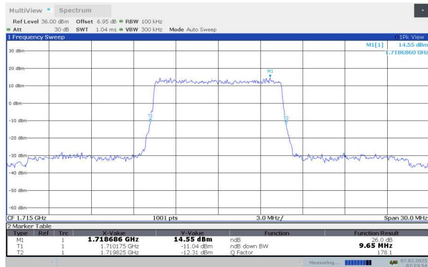
**LTE Band 66 , 10MHz Bandwidth,LOW,16QAM (-26dBc OBW)**
