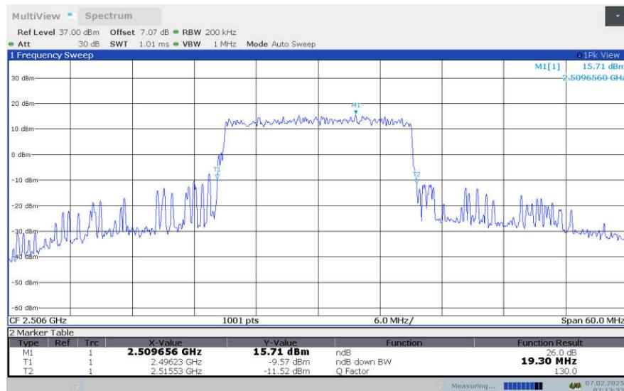
**LTE Band 41 , 20MHz Bandwidth,LOW,64QAM (-26dBc OBW)**
