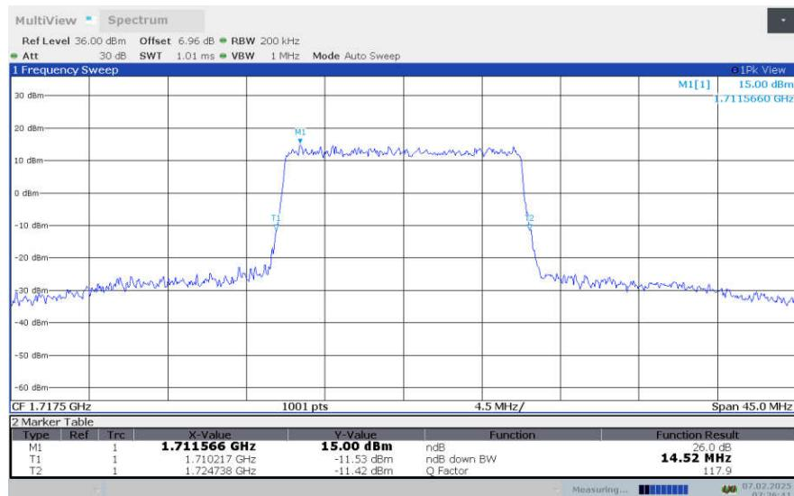
**LTE Band 66 , 15MHz Bandwidth,LOW,64QAM (-26dBc OBW)**
