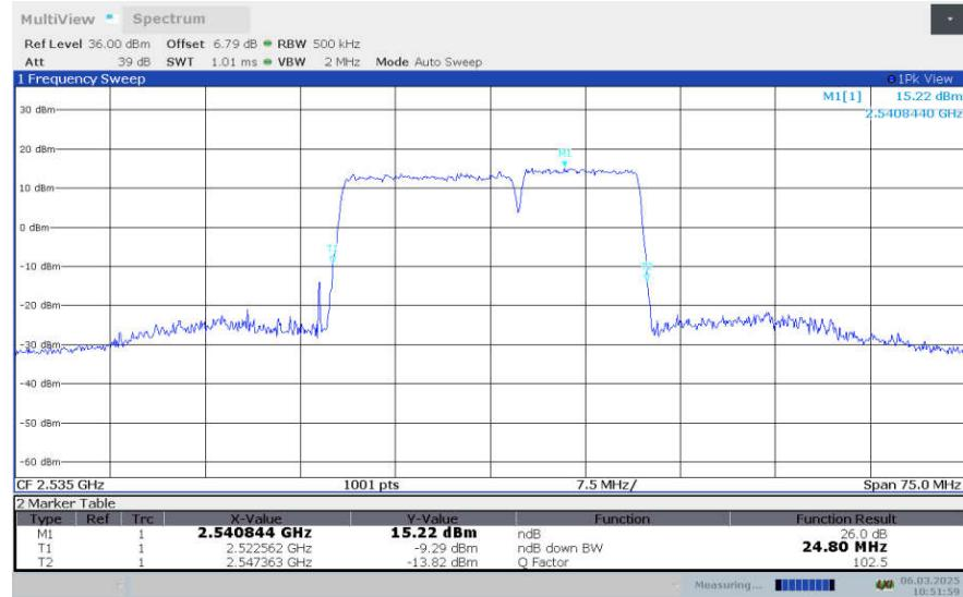
**LTE CA\_7C , 15MHz+10MHz Bandwidth,16QAM (-26dBc OBW)**
