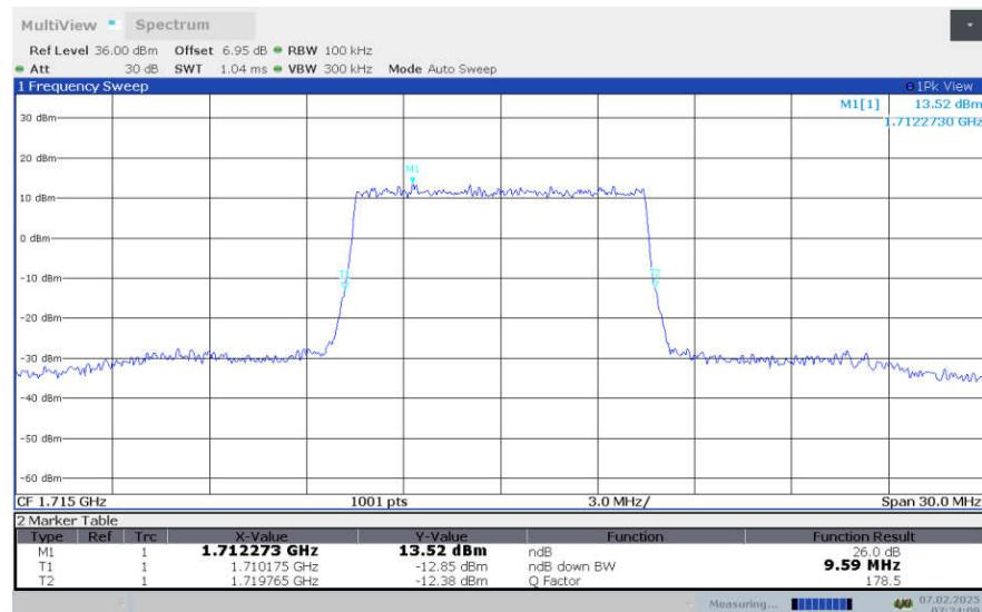
**LTE Band 66 , 10MHz Bandwidth,LOW,64QAM (-26dBc OBW)**
