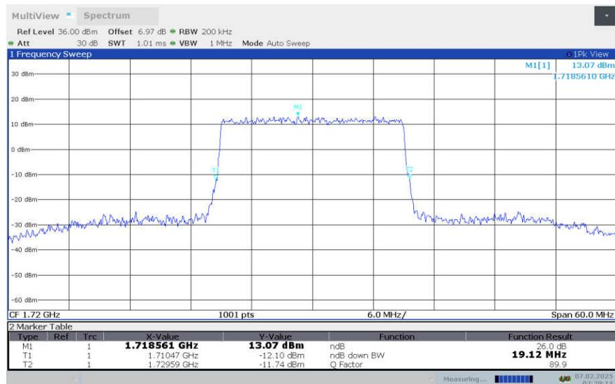
**LTE Band 66 , 20MHz Bandwidth,LOW,64QAM (-26dBc OBW)**
