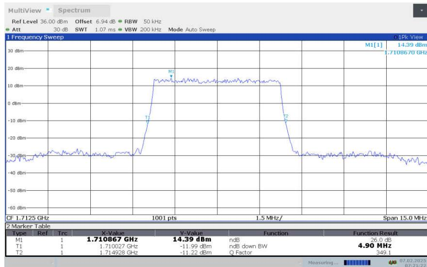
**LTE Band 66 , 5MHz Bandwidth,LOW,16QAM (-26dBc OBW)**
