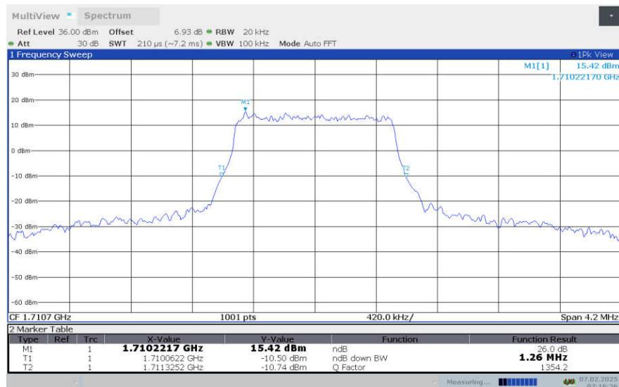
**LTE Band 66 , 1.4MHz Bandwidth,LOW,64QAM (-26dBc OBW)**
