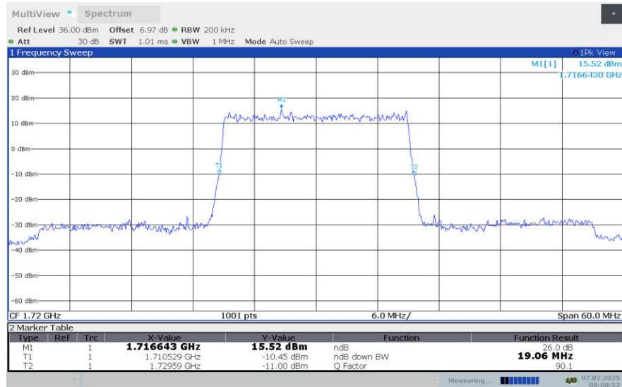
**LTE Band 66 , 20MHz Bandwidth,LOW,16QAM (-26dBc OBW)**
