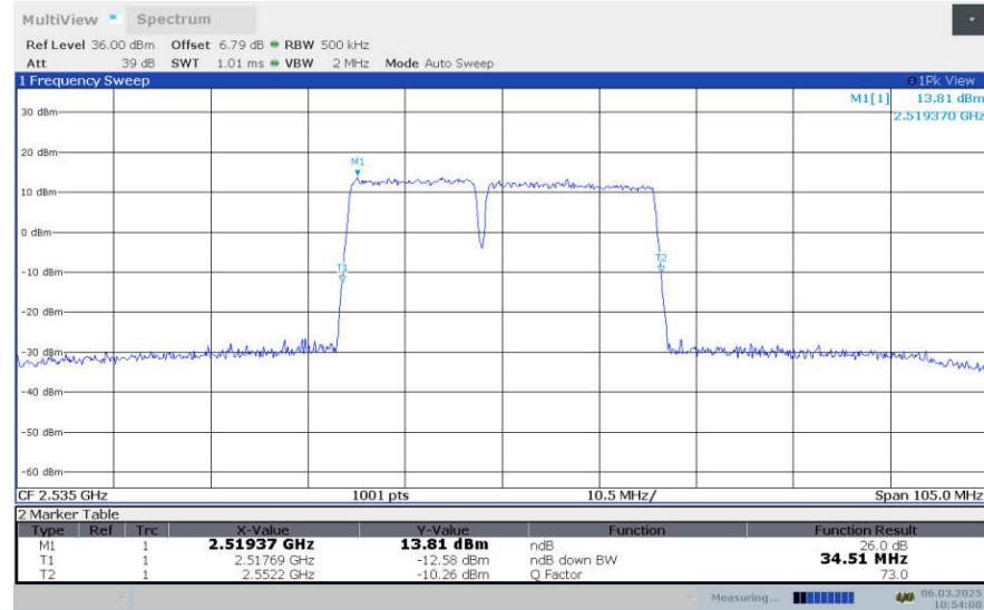
**LTE CA\_7C , 15MHz+20MHz Bandwidth,16QAM (-26dBc OBW)**
