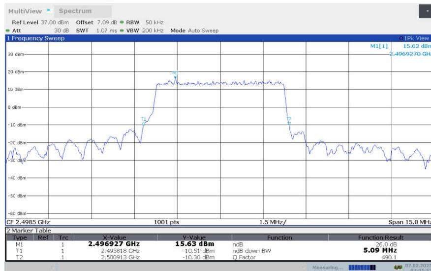
**LTE Band 41 , 5MHz Bandwidth,LOW,64QAM (-26dBc OBW)**
