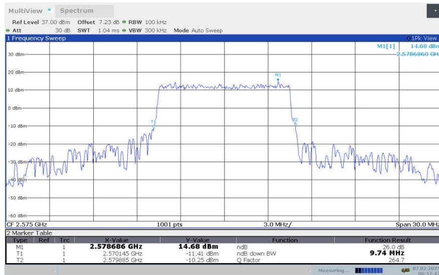
**LTE Band 38 , 10MHz Bandwidth,LOW,16QAM (-26dBc OBW)**
