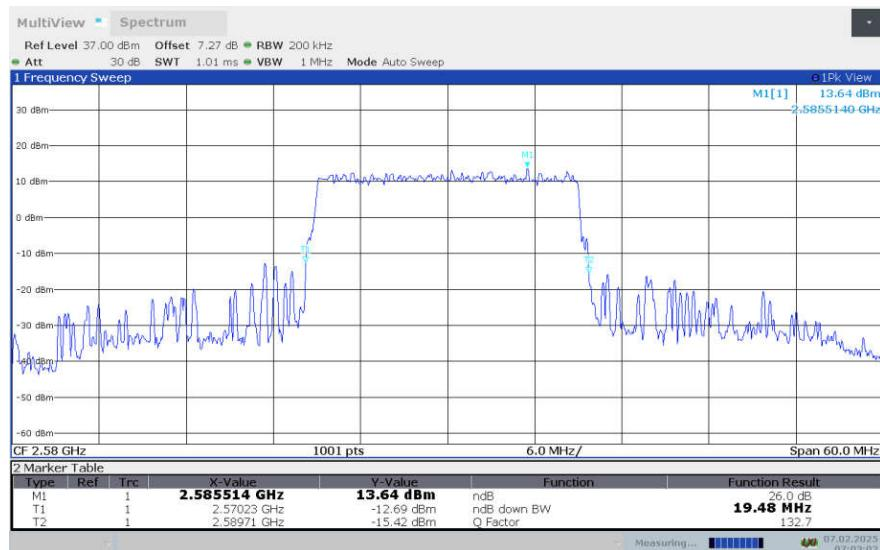
**LTE Band 38 , 20MHz Bandwidth,LOW,64QAM (-26dBc OBW)**
