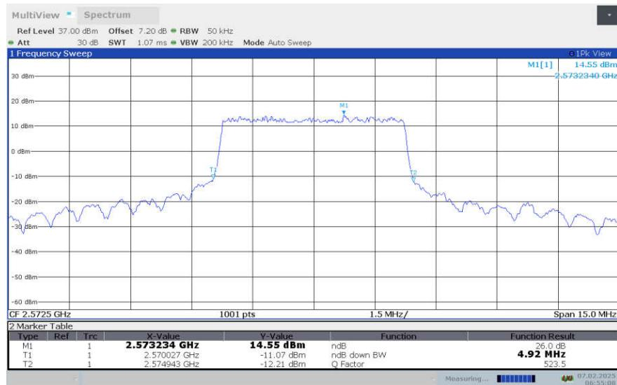
**LTE Band 38 , 5MHz Bandwidth,LOW,16QAM (-26dBc OBW)**
