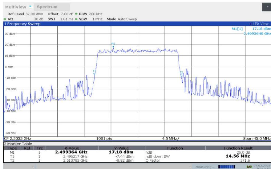
**LTE Band 41 , 15MHz Bandwidth,LOW,64QAM (-26dBc OBW)**
