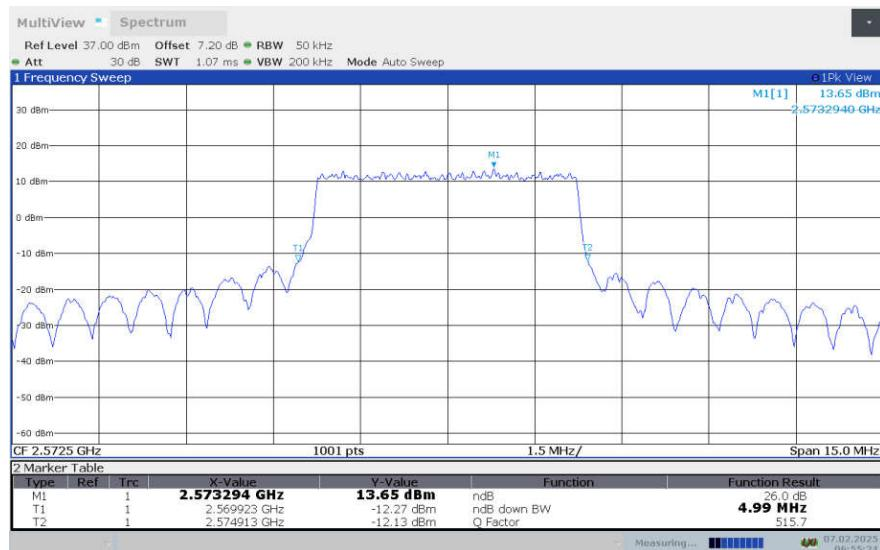
**LTE Band 38 , 5MHz Bandwidth,LOW,64QAM (-26dBc OBW)**
