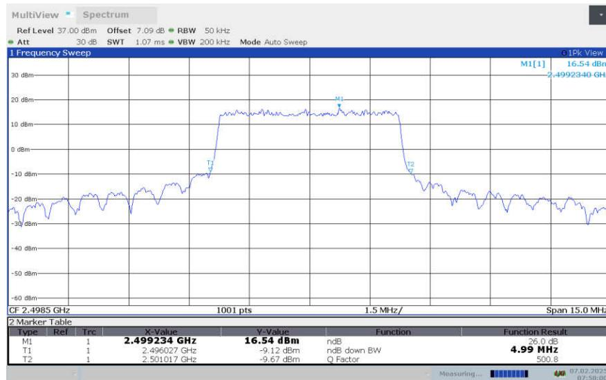
**LTE Band 41 , 5MHz Bandwidth,LOW,16QAM (-26dBc OBW)**
