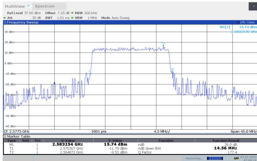
**LTE Band 38 , 15MHz Bandwidth,LOW,16QAM (-26dBc OBW)**
