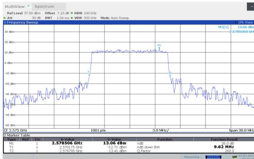
**LTE Band 38 , 10MHz Bandwidth,LOW,64QAM (-26dBc OBW)**
