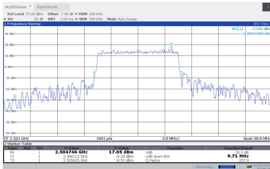
**LTE Band 41 , 10MHz Bandwidth,LOW,64QAM (-26dBc OBW)**
