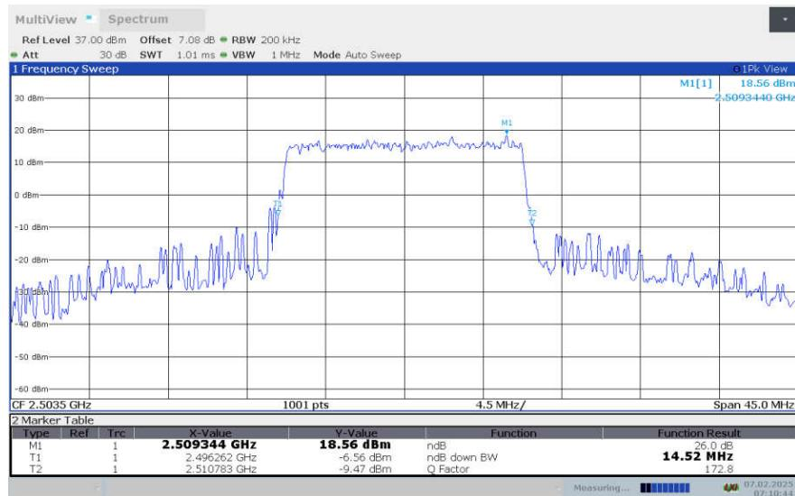
**LTE Band 41 , 15MHz Bandwidth,LOW,16QAM (-26dBc OBW)**
