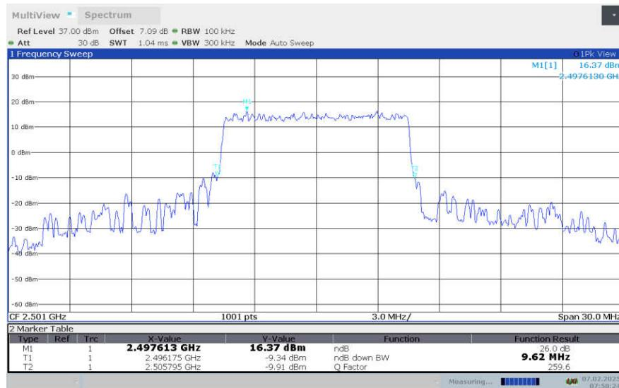
**LTE Band 41 , 10MHz Bandwidth,LOW,16QAM (-26dBc OBW)**
