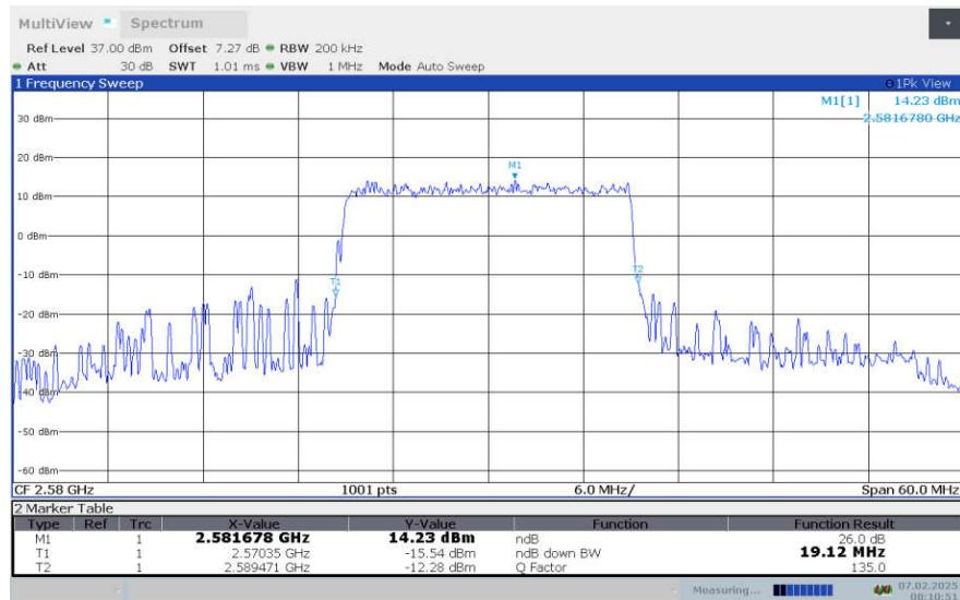
**LTE Band 38 , 20MHz Bandwidth,LOW,16QAM (-26dBc OBW)**
