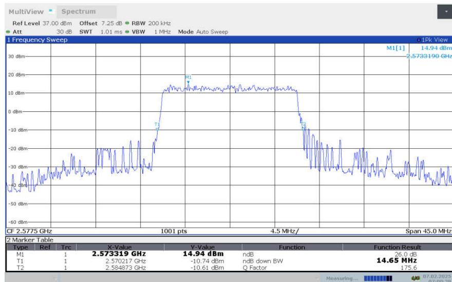
**LTE Band 38 , 15MHz Bandwidth,LOW,64QAM (-26dBc OBW)**
