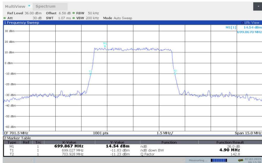
**LTE Band 12,5MHz Bandwidth,LOW,16QAM (-26dBc OBW)**
