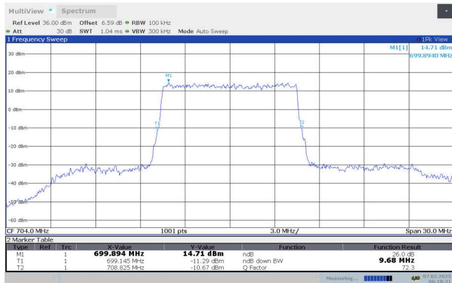
**LTE Band 12 , 10MHz Bandwidth,LOW,16QAM (-26dBc OBW)**
