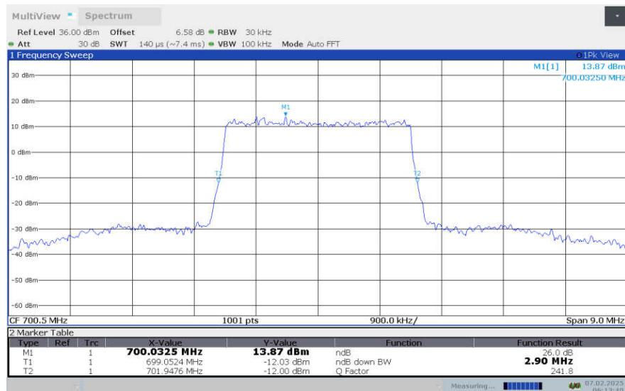
**LTE Band 12, 3MHz Bandwidth,LOW,64QAM (-26dBc OBW)**
