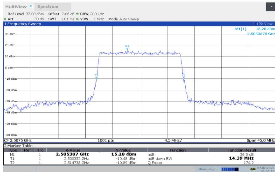
**LTE Band 7 , 15MHz Bandwidth,LOW,16QAM (-26dBc OBW)**
