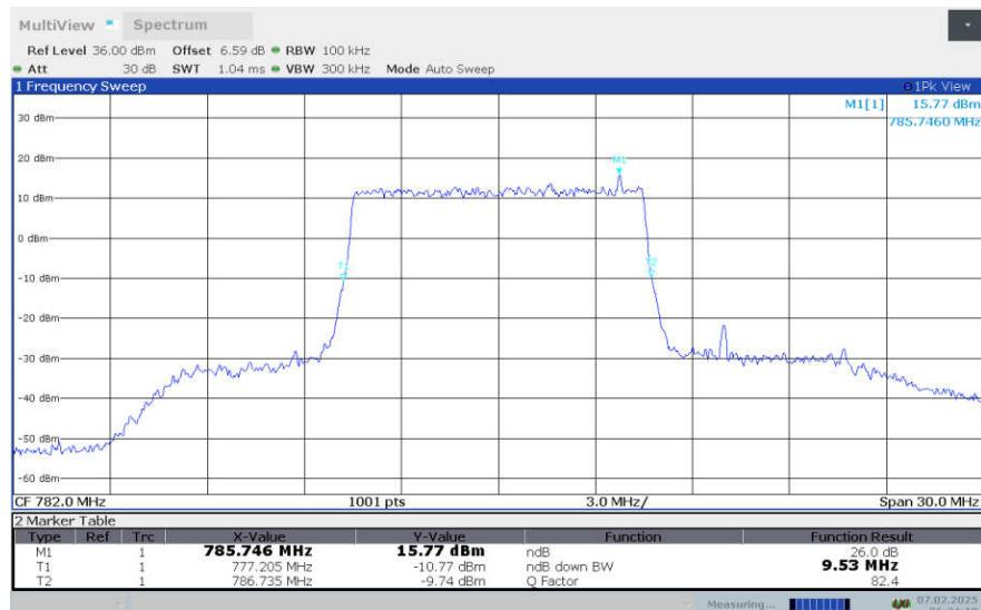
**LTE Band 13 , 10MHz Bandwidth,LOW,64QAM (-26dBc OBW)**
