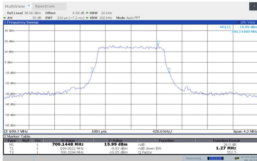
**LTE Band 12, 1.4MHz Bandwidth,LOW,16QAM (-26dBc OBW)**
