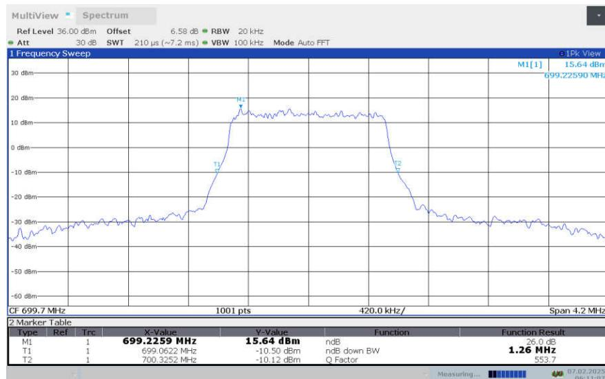
**LTE Band 12, 1.4MHz Bandwidth,LOW,64QAM (-26dBc OBW)**
