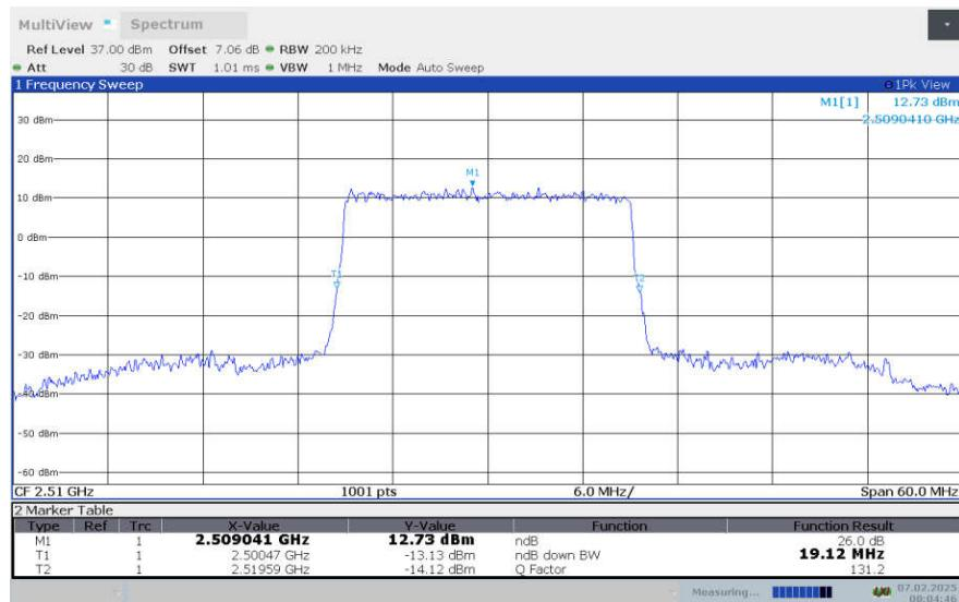
**LTE Band 7 , 20MHz Bandwidth,LOW,64QAM (-26dBc OBW)**
