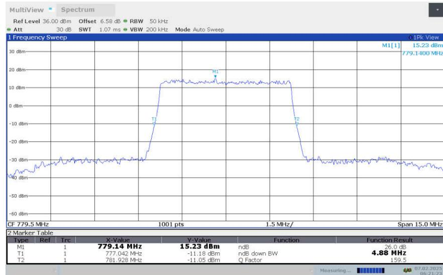
**LTE Band 13 , 5MHz Bandwidth,LOW,16QAM (-26dBc OBW)**
