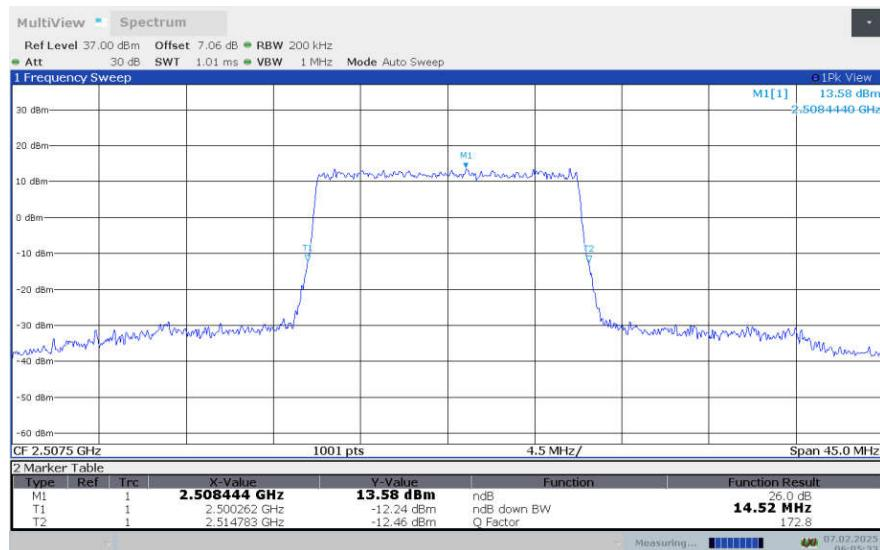
**LTE Band 7 , 15MHz Bandwidth,LOW,64QAM (-26dBc OBW)**
