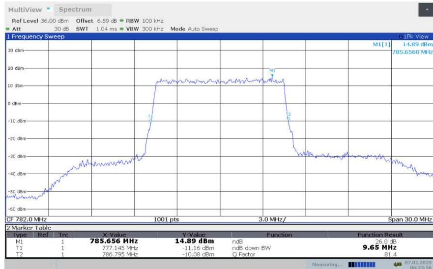
**LTE Band 13 , 10MHz Bandwidth,LOW,16QAM (-26dBc OBW)**
