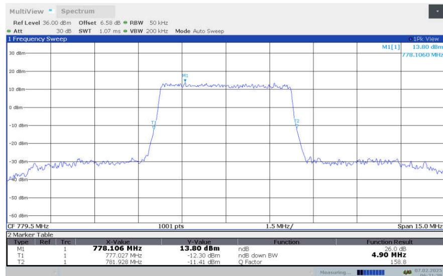
**LTE Band 13 , 5MHz Bandwidth,LOW,64QAM (-26dBc OBW)**
