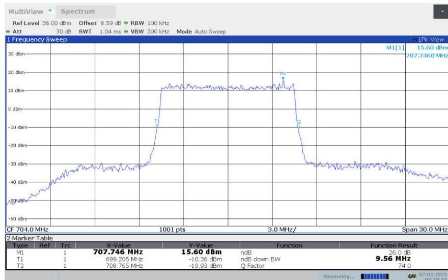
**LTE Band 12 , 10MHz Bandwidth,LOW,64QAM (-26dBc OBW)**
