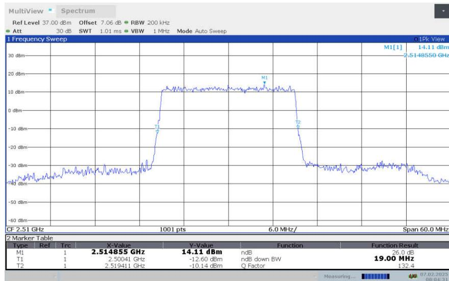
**LTE Band 7 , 20MHz Bandwidth,LOW,16QAM (-26dBc OBW)**
