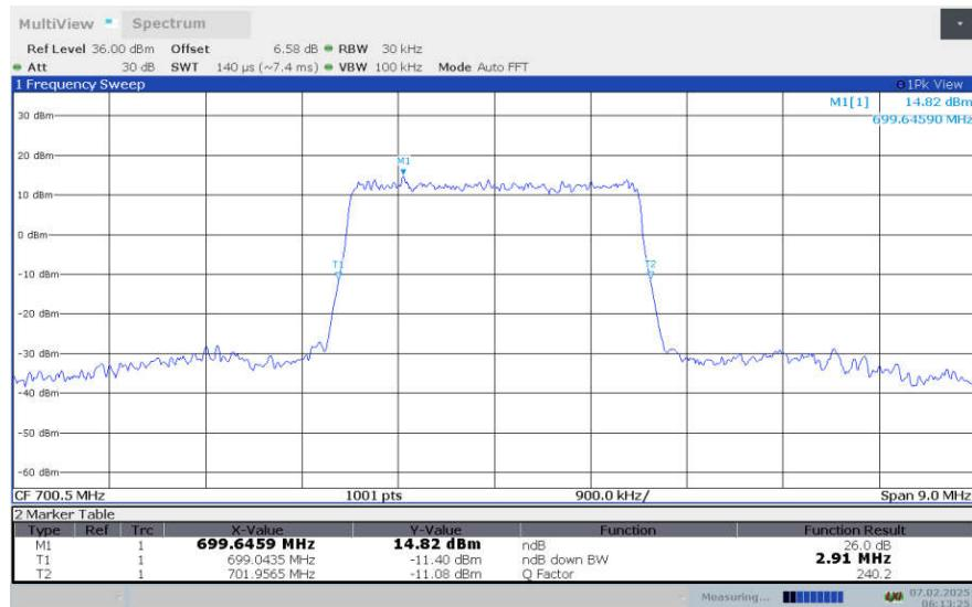
**LTE Band 12, 3MHz Bandwidth,LOW,16QAM (-26dBc OBW)**
