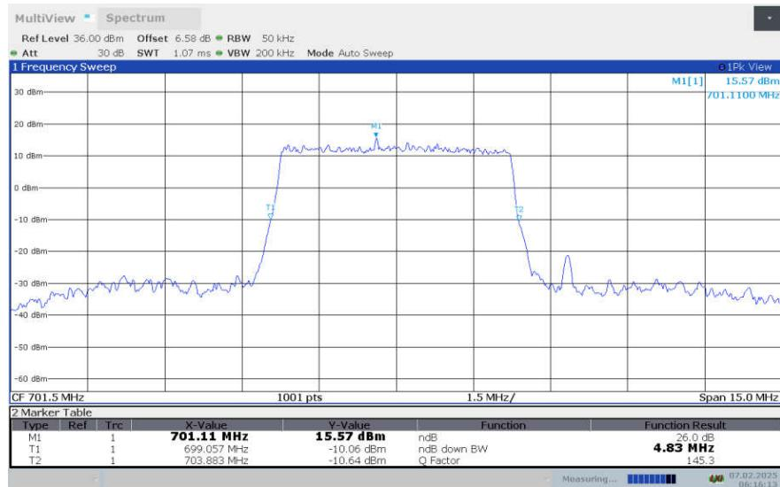
**LTE Band 12,5MHz Bandwidth,LOW,64QAM (-26dBc OBW)**
