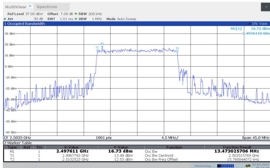
**LTE Band 41 , 15MHz Bandwidth,LOW,64QAM (99% OBW)**
