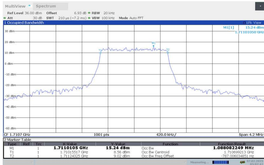
**LTE Band 66, 1.4MHz Bandwidth,LOW,64QAM (99% OBW)**
