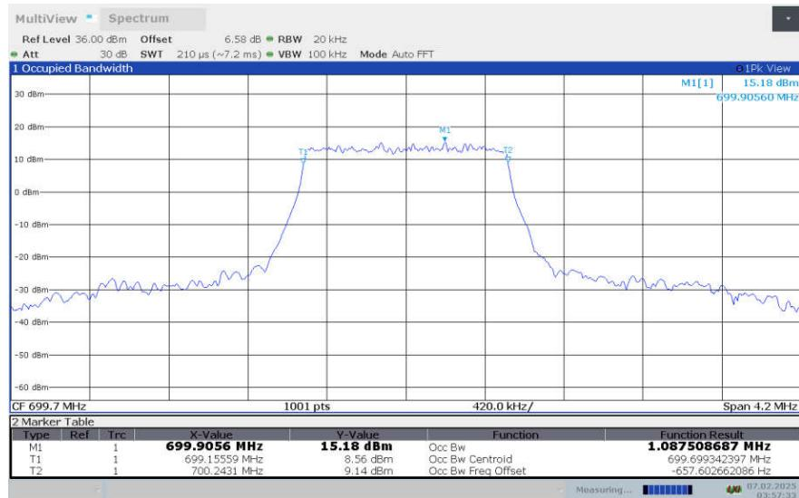
**LTE Band 12, 1.4MHz Bandwidth,LOW,64QAM (99% OBW)**
