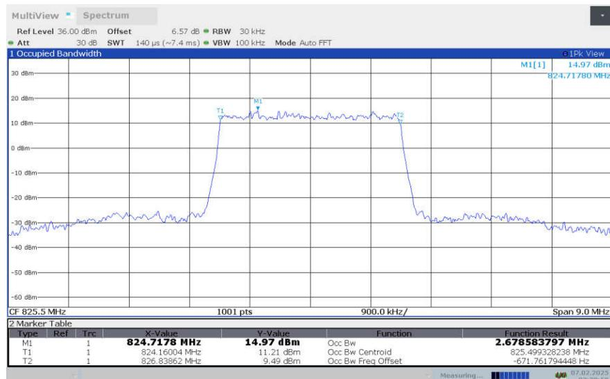
**LTE Band 5, 3MHz Bandwidth,LOW,64QAM (99% OBW)**
