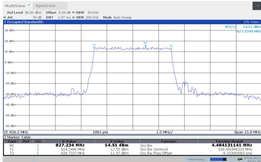
**LTE Band 5, 5MHz Bandwidth, LOW, 16QAM (99% OBW)**
