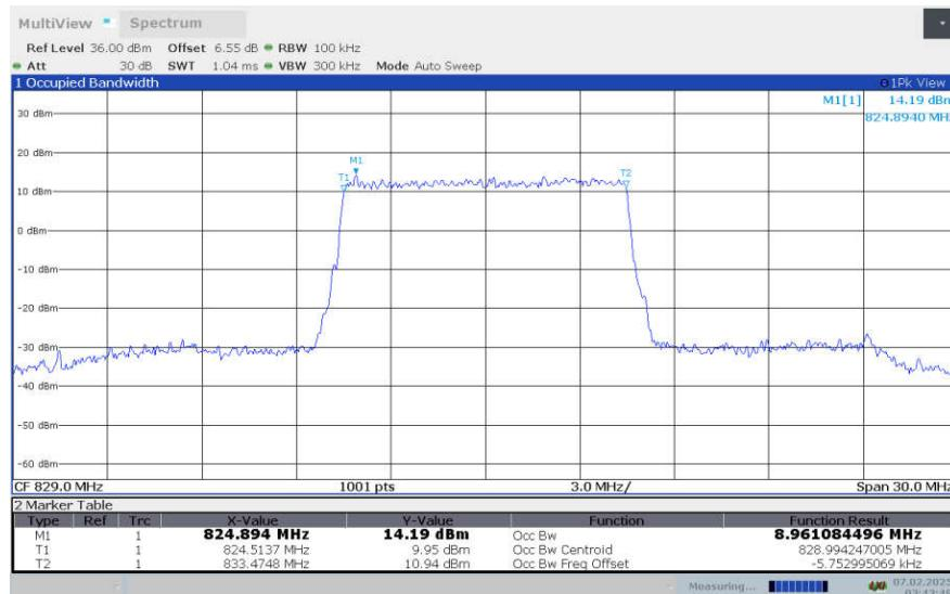
**LTE Band 5, 10MHz Bandwidth,LOW,16QAM (99% OBW)**
