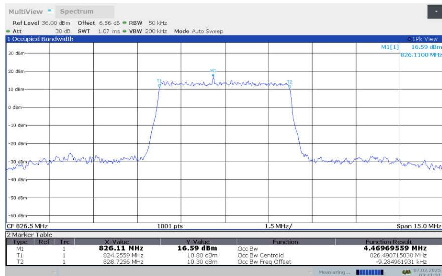
**LTE Band 5, 5MHz Bandwidth, LOW, 64QAM (99% OBW)**
