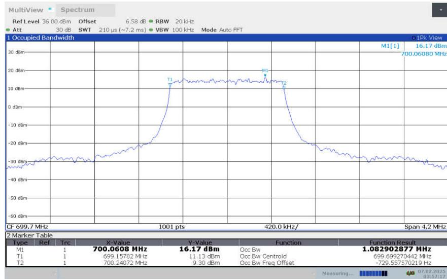
**LTE Band 12, 1.4MHz Bandwidth,LOW,16QAM (99% OBW)**
