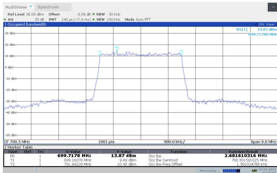
**LTE Band 12, 3MHz Bandwidth,LOW,64QAM (99% OBW)**
