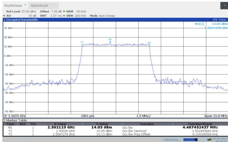
**LTE Band 7, 5MHz Bandwidth,LOW,16QAM (99% OBW)**
