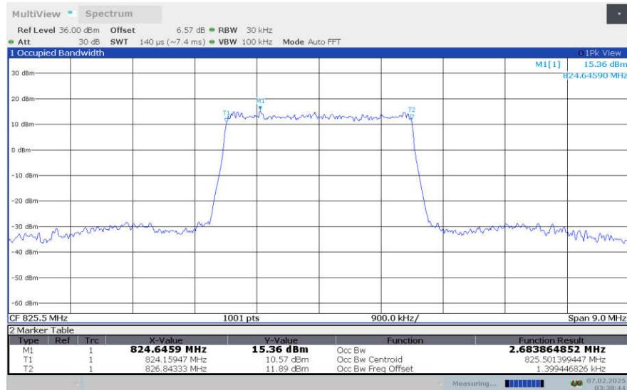
**LTE Band 5, 3MHz Bandwidth,LOW,16QAM (99% OBW)**
