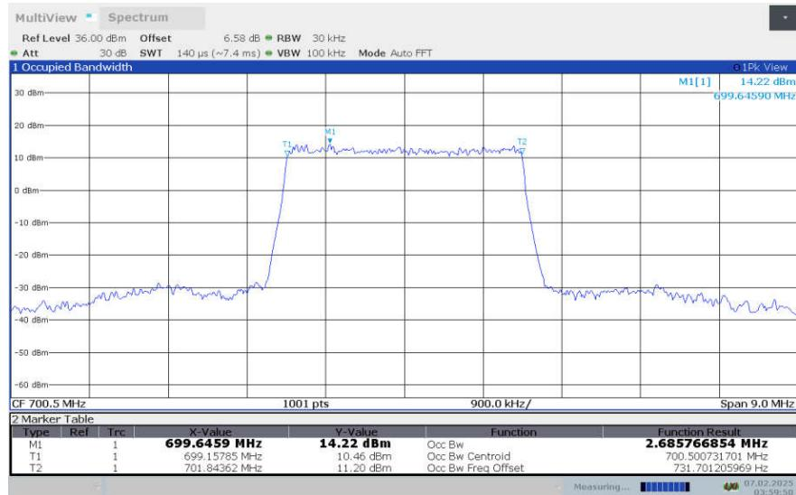
**LTE Band 12, 3MHz Bandwidth,LOW,16QAM (99% OBW)**
