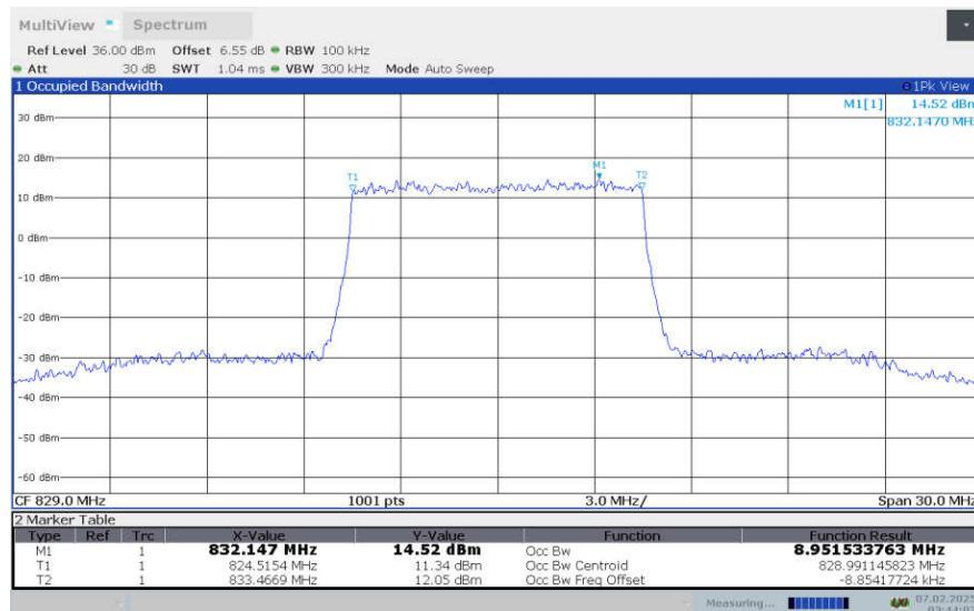
**LTE Band 5, 10MHz Bandwidth,LOW,64QAM (99% OBW)**
