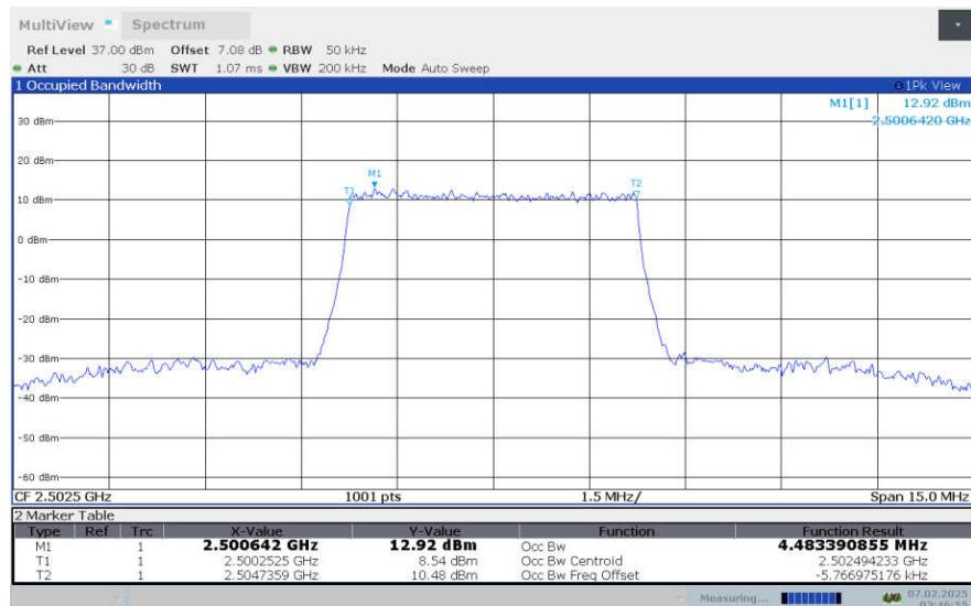
**LTE Band 7, 5MHz Bandwidth,LOW,64QAM (99% OBW)**
