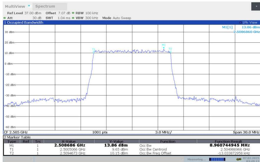
**LTE Band 7 , 10MHz Bandwidth,LOW,16QAM (99% OBW)**
