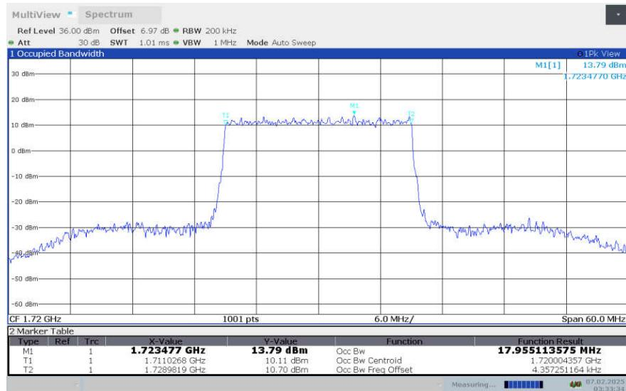
**LTE Band 4, 20MHz Bandwidth,LOW,64QAM (99% OBW)**
