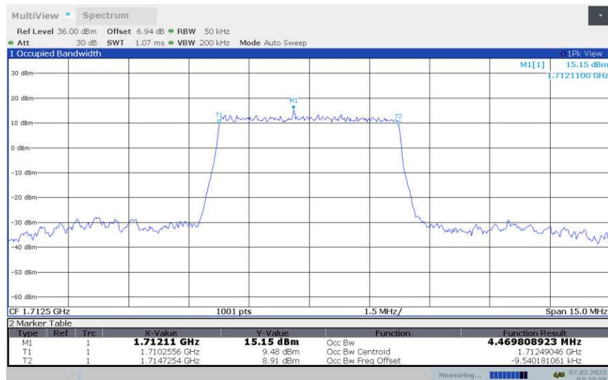
**LTE Band 4, 5MHz Bandwidth,LOW,64QAM (99% OBW)**
