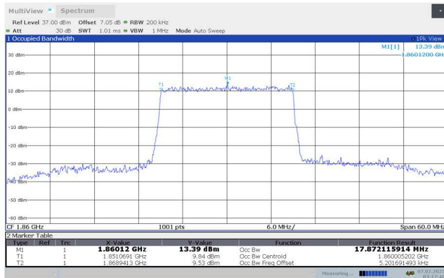
**LTE Band 2, 20MHz Bandwidth,LOW,16QAM (99% OBW)**
