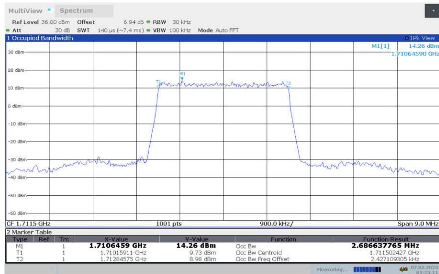
**LTE Band 4, 3MHz Bandwidth, LOW, 16QAM (99% OBW)**
