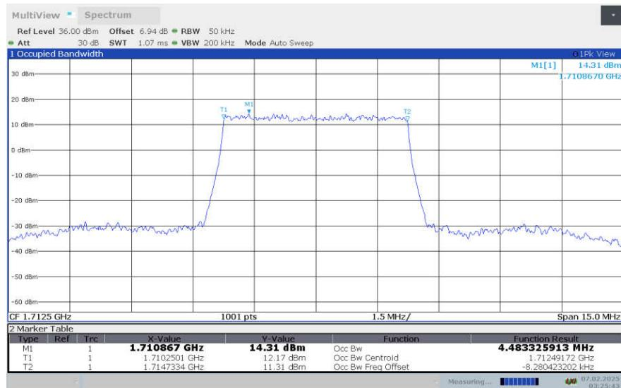
**LTE Band 4, 5MHz Bandwidth,LOW,16QAM (99% OBW)**
