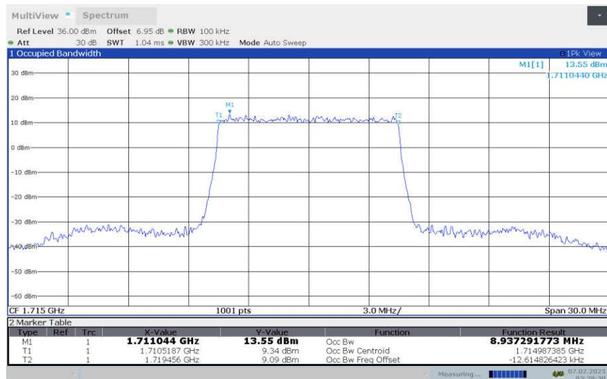
**LTE Band 4, 10MHz Bandwidth,LOW,64QAM (99% OBW)**
