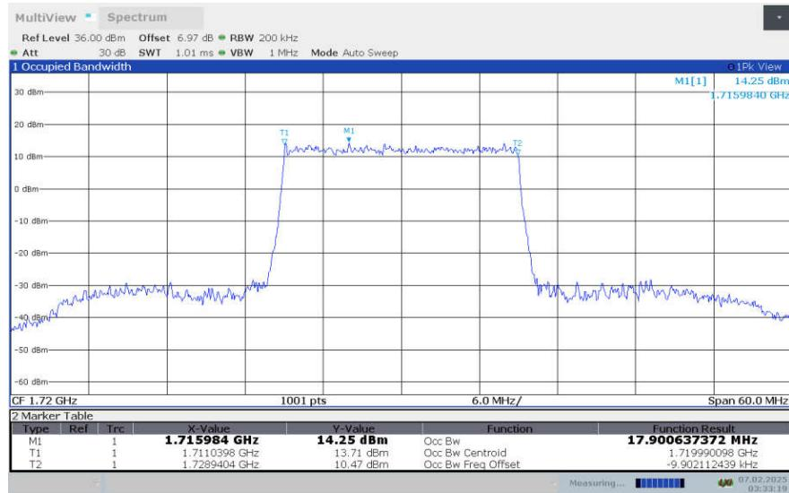
**LTE Band 4, 20MHz Bandwidth,LOW,16QAM (99% OBW)**
