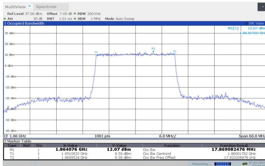
**LTE Band 2, 20MHz Bandwidth,LOW,64QAM (99% OBW)**
