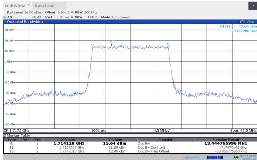
**LTE Band 4, 15MHz Bandwidth,LOW,16QAM (99% OBW)**
