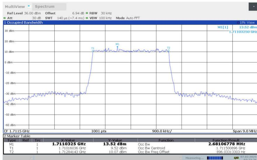
**LTE Band 4, 3MHz Bandwidth, LOW, 64QAM (99% OBW)**
