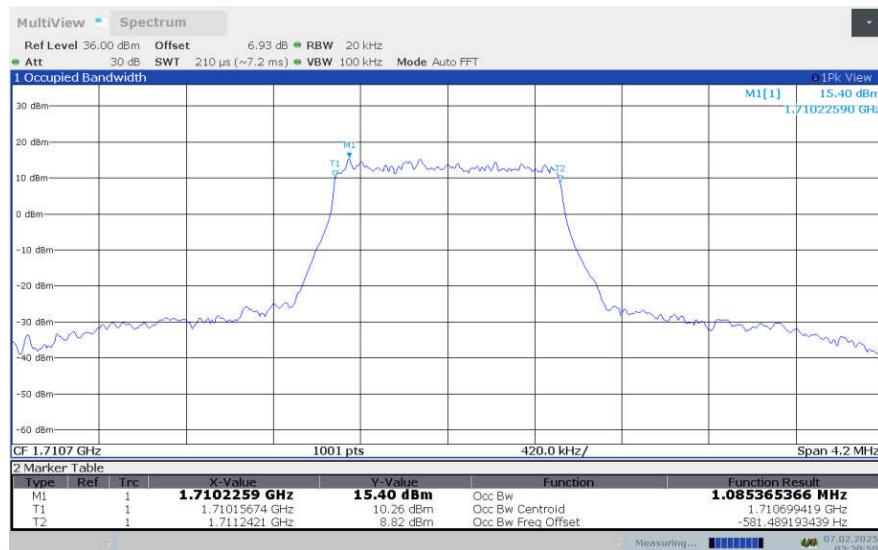
**LTE Band 4, 1.4MHz Bandwidth,LOW,64QAM (99% OBW)**
