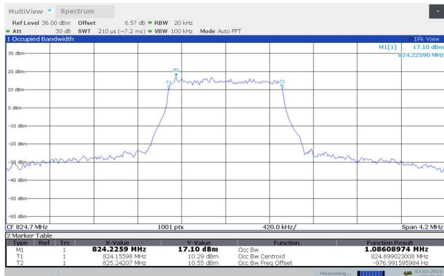
**LTE Band 5, 1.4MHz Bandwidth,LOW,64QAM (99% OBW)**
