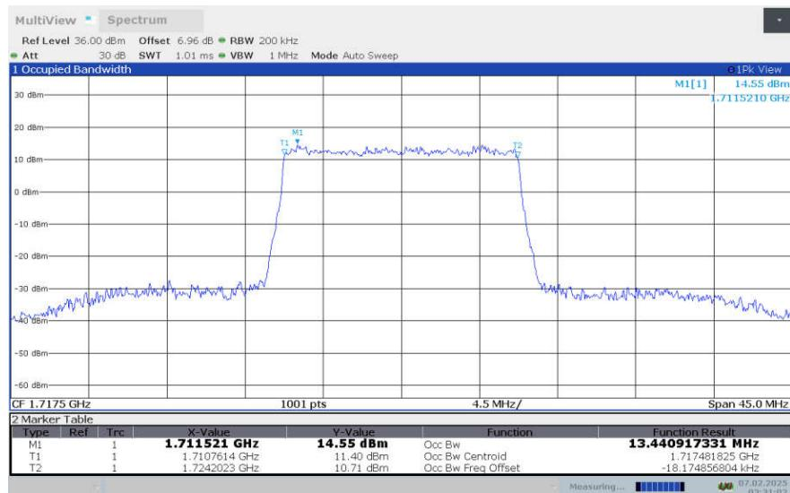
**LTE Band 4, 15MHz Bandwidth,LOW,64QAM (99% OBW)**
