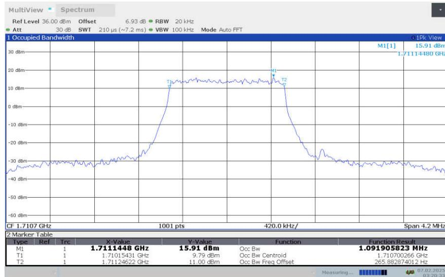
**LTE Band 4, 1.4MHz Bandwidth,LOW,16QAM (99% OBW)**
