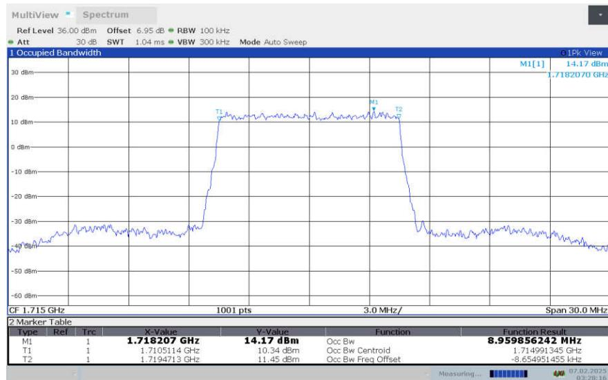
**LTE Band 4, 10MHz Bandwidth,LOW,16QAM (99% OBW)**
