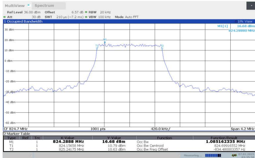
**LTE Band 5, 1.4MHz Bandwidth,LOW,16QAM (99% OBW)**
