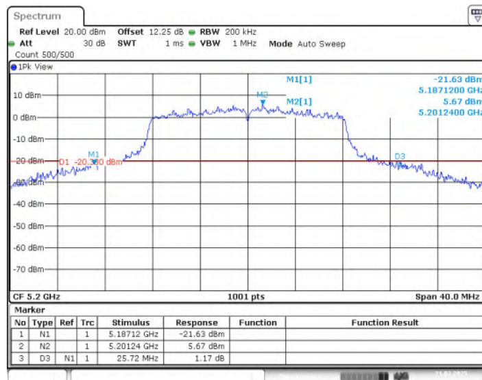
Fig. 2 Occupied 26dB Bandwidth (802.11a, 5200MHz)
