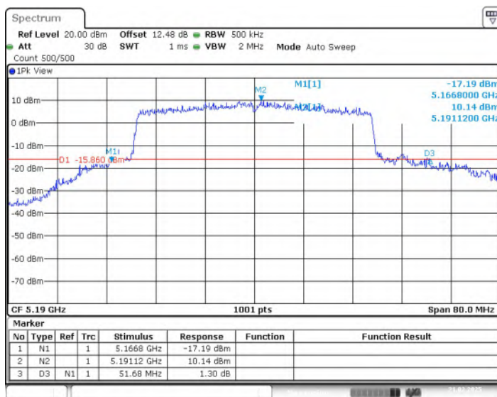
Fig. 3 Occupied 26dB Bandwidth (802.11ax-HE40, 5190MHz)
