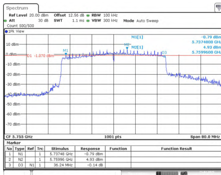
Fig. 12 Occupied 6dB Bandwidth (802.11ax-HE40, 5755MHz)
