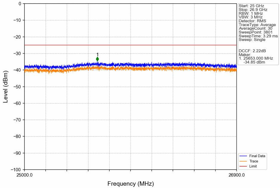
CA\_41C\_SISO\_NTNV\_CC1:5 CC2:20MHz\_CC1:64QAM CC2:64QAM\_CC1:2668.3 CC2:2680MHz\_CC1: 1@0 CC2: 1@0
