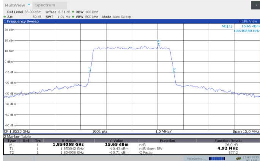
**n2,5MHz Bandwidth,DFT-s-64QAM (-26dBc OBW)**
