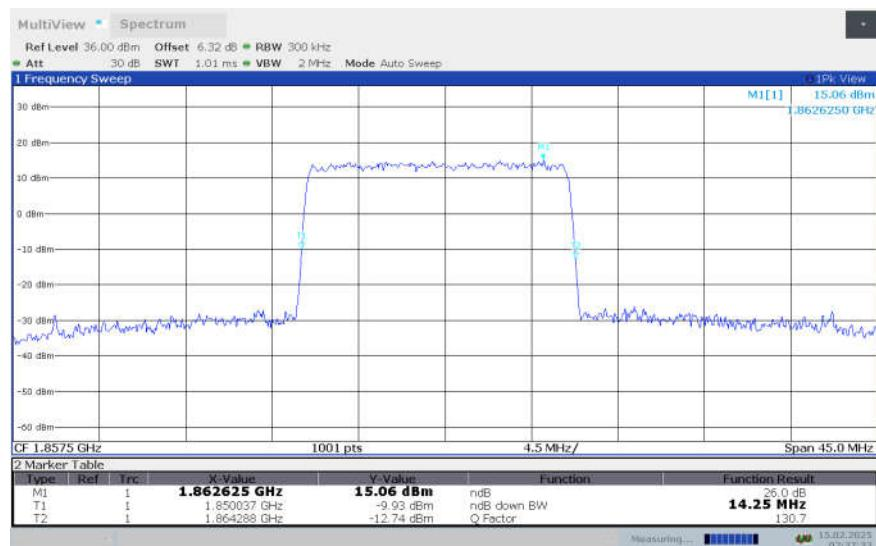
**n2,15MHz Bandwidth,DFT-s-16QAM (-26dBc OBW)**
