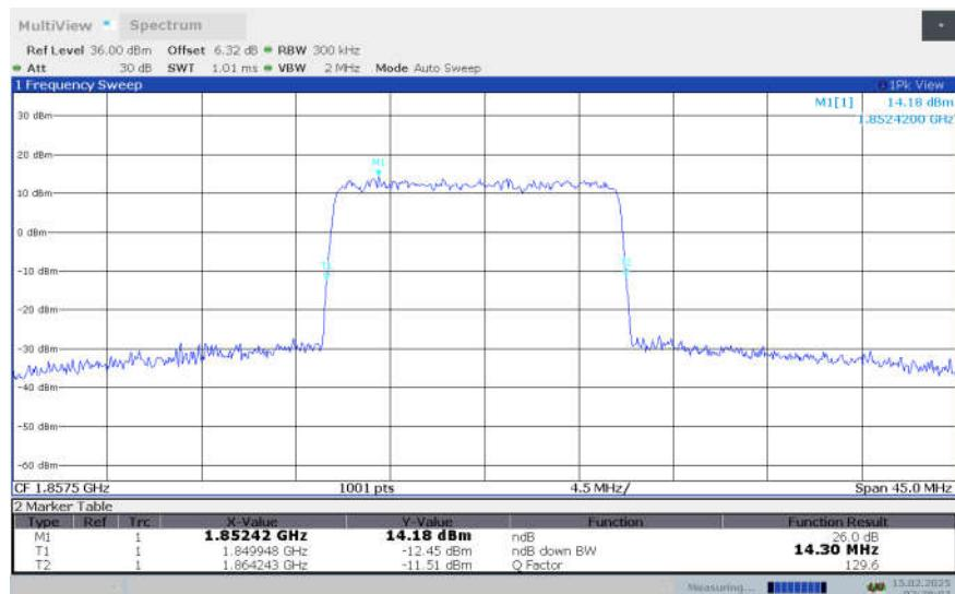
**n2,15MHz Bandwidth,DFT-s-256QAM (-26dBc OBW)**
