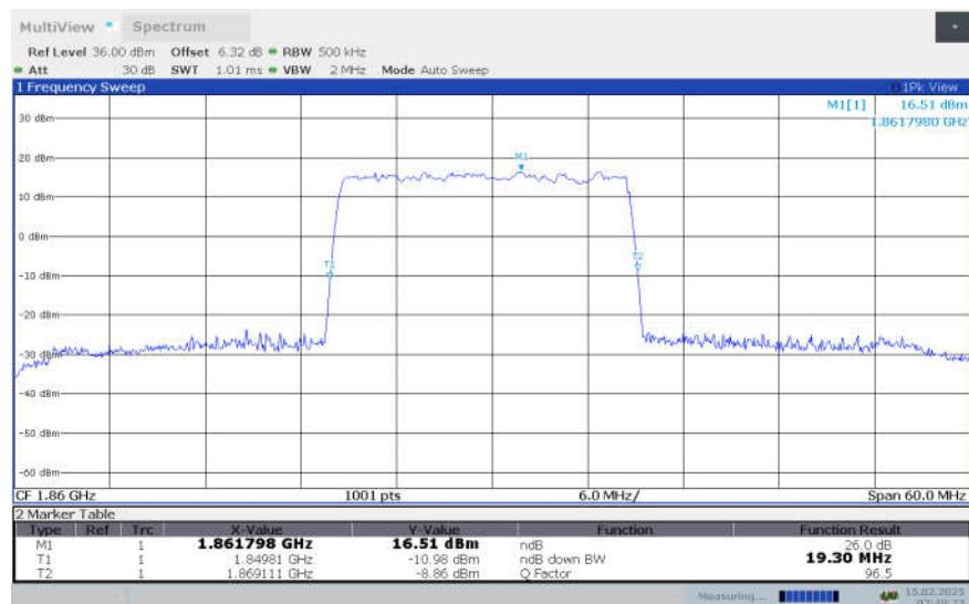
**n2,20MHz Bandwidth,DFT-s-16QAM (-26dBc OBW)**
