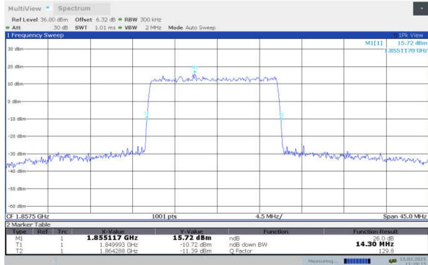
**n2,15MHz Bandwidth,DFT-s-64QAM (-26dBc OBW)**
