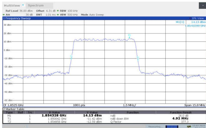
**n2,5MHz Bandwidth,DFT-s-256QAM (-26dBc OBW)**
