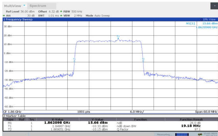
**n2,20MHz Bandwidth,DFT-s-256QAM (-26dBc OBW)**
