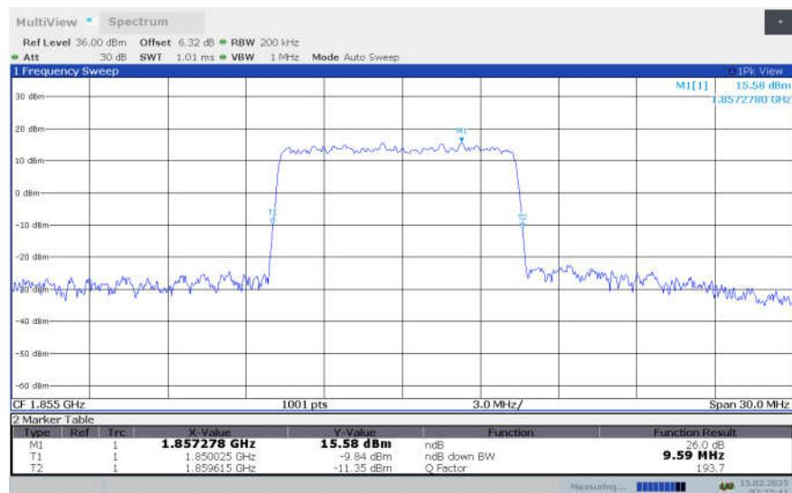
**n2,10MHz Bandwidth,DFT-s-16QAM (-26dBc OBW)**
