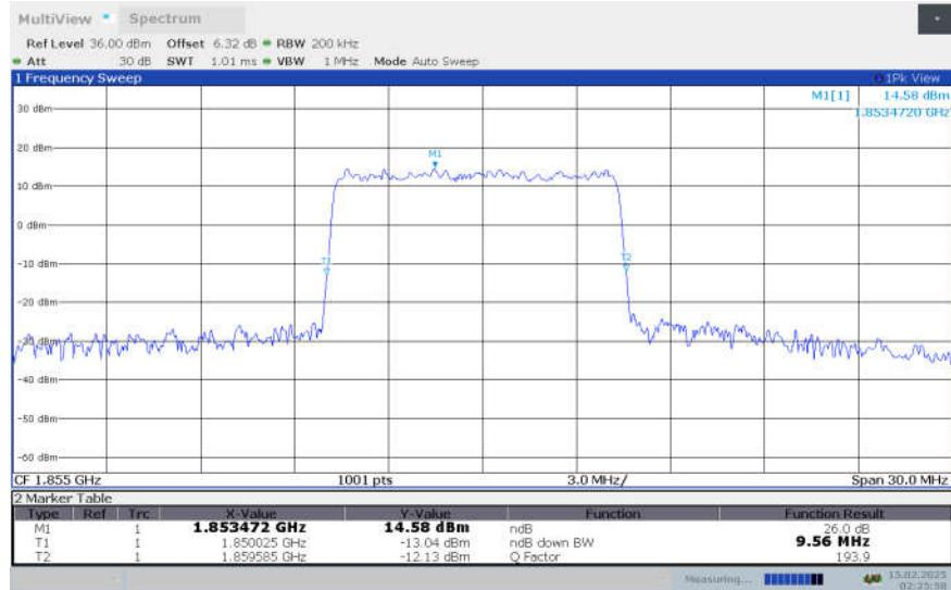
**n2,10MHz Bandwidth,DFT-s-64QAM (-26dBc OBW)**
