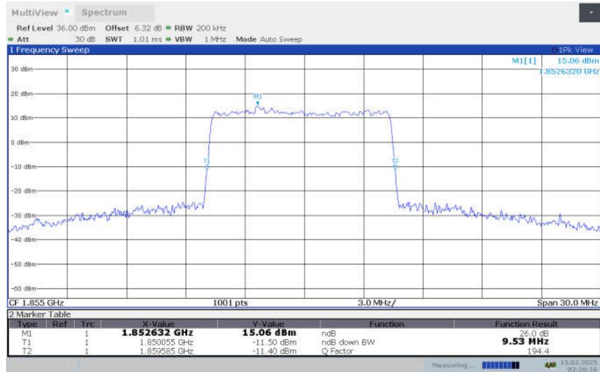
**n2,10MHz Bandwidth,DFT-s-256QAM (-26dBc OBW)**
