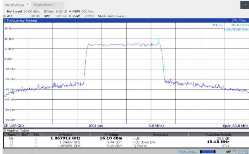
**n2,20MHz Bandwidth,DFT-s-64QAM (-26dBc OBW)**
