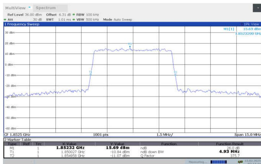
**n2,5MHz Bandwidth,DFT-s-16QAM (-26dBc OBW)**
