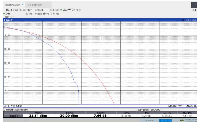
**LTE Band 66 , 3MHz Bandwidth,64QAM**
