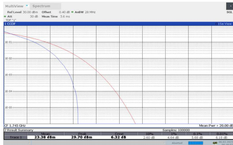
**LTE Band 66 , 3MHz Bandwidth,16QAM**
